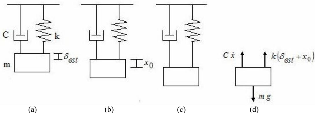
**Figure 1. (a) mass/damper/spring system, (b) static equilibrium displacement, (c) adding initial non-equilibrium displacement and (d) free body diagram of last position.**
