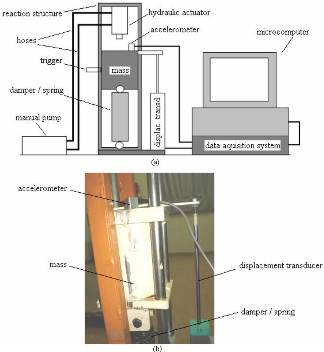
Figure 2. (a) Schematic view of experiment and (b) detailed view of experiment.
