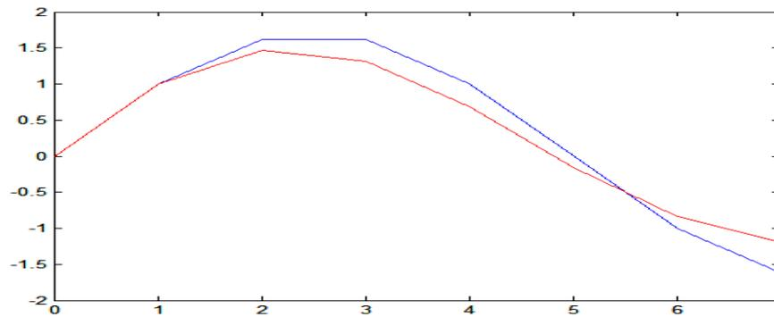
Figure 3. Second mode shape (blue line: exact mode shape and red line: identified mode)
