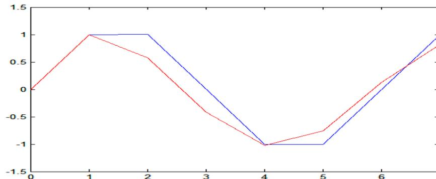
Figure 4. Third mode shape (blue line: exact mode shape and red line: identified mode)
