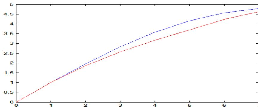
Figure 2. First mode shape (blue line: exact mode shape and red line: identified mode)
