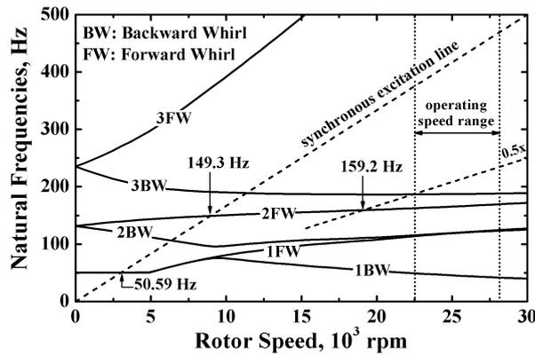
Figure 5. Campbell diagram of the studied rotor-bearing system.
