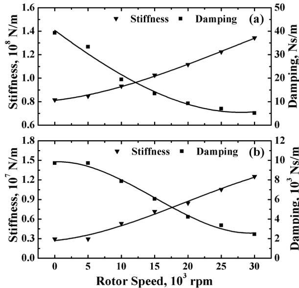
Figure 3. Dynamic coefficients of the bearings: (a) a lubricated deep groove ball bearing (front bearing) and (b) a squeeze film damper (rear bearing).
