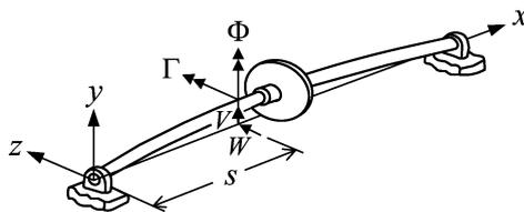
Figure 2. Displacement variables and coordinate system of a rotor-bearing system.
