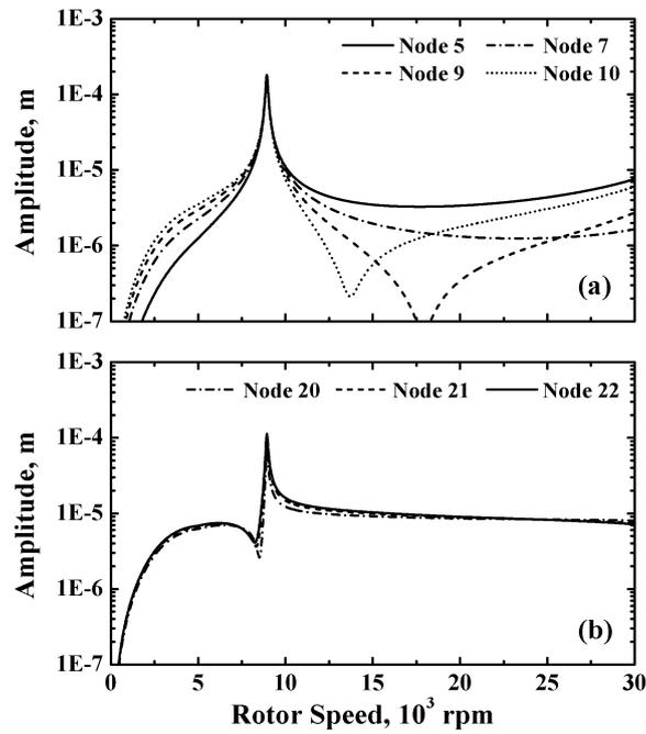
Figure 7. Unbalance responses at specific nodes of the model: (a) nodes of the five-stage axial compressor and (b) nodes of the free turbine rotor.
