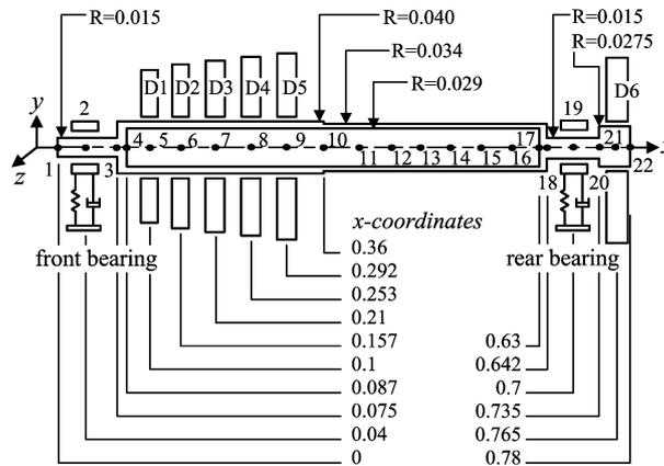
Figure 4. Rotor-bearing model of the studied gas turbine. All dimensions are in meters.
