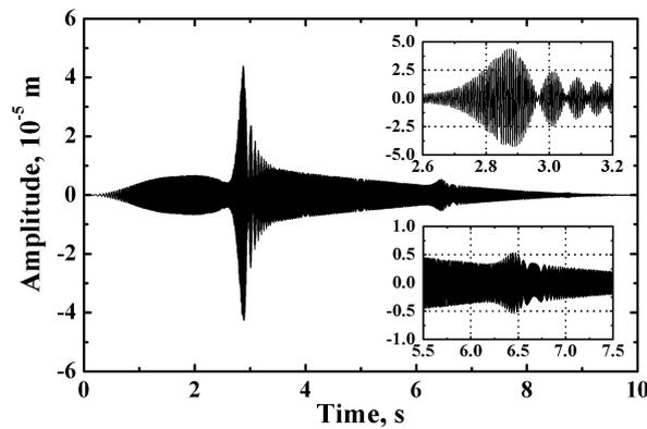
Figure 8. Transition of the studied rotor-bearing system through resonance. The displacements are evaluated in the y-direction at node 21.
