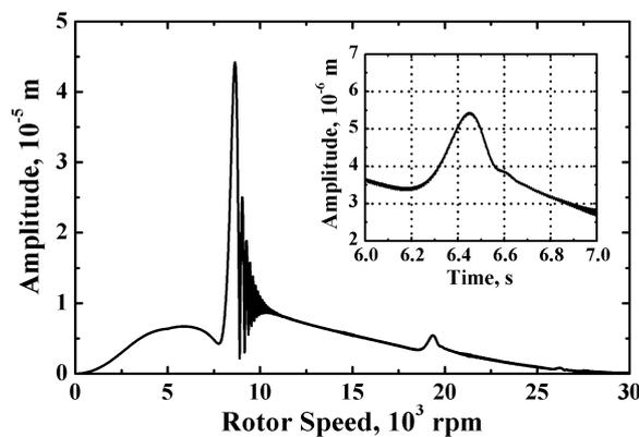
Figure 9. Total displacements at node 21 during transition of the system through resonance.
