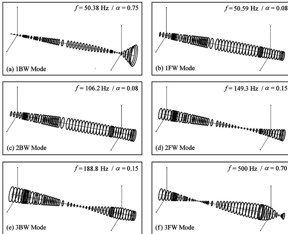
Figure 6. Modal orbits of the shaft plotted at the critical frequencies of the system with respect to the synchronous excitation line. The parameter  $\alpha$  is a scale-view factor.
