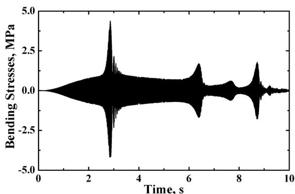
Figure 10. Bending stresses evaluated at node 20 during system transition through resonance.
