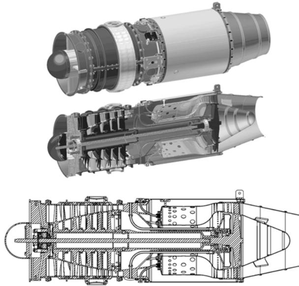
Figure 1. Cross-section view of the studied single spool gas turbine.
