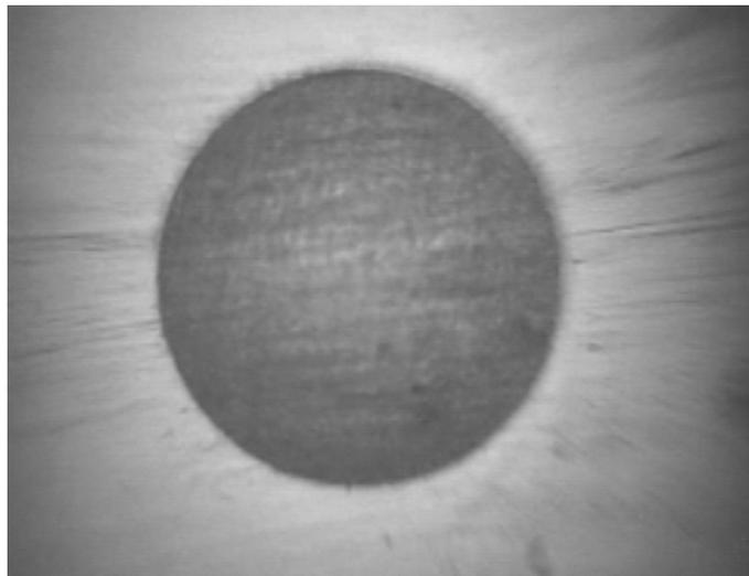
Illustration 3. Photo of the crater obtained in the *Test of micro Abrasion Ball Cratering*, optical microscope, magnified by 80 x.
