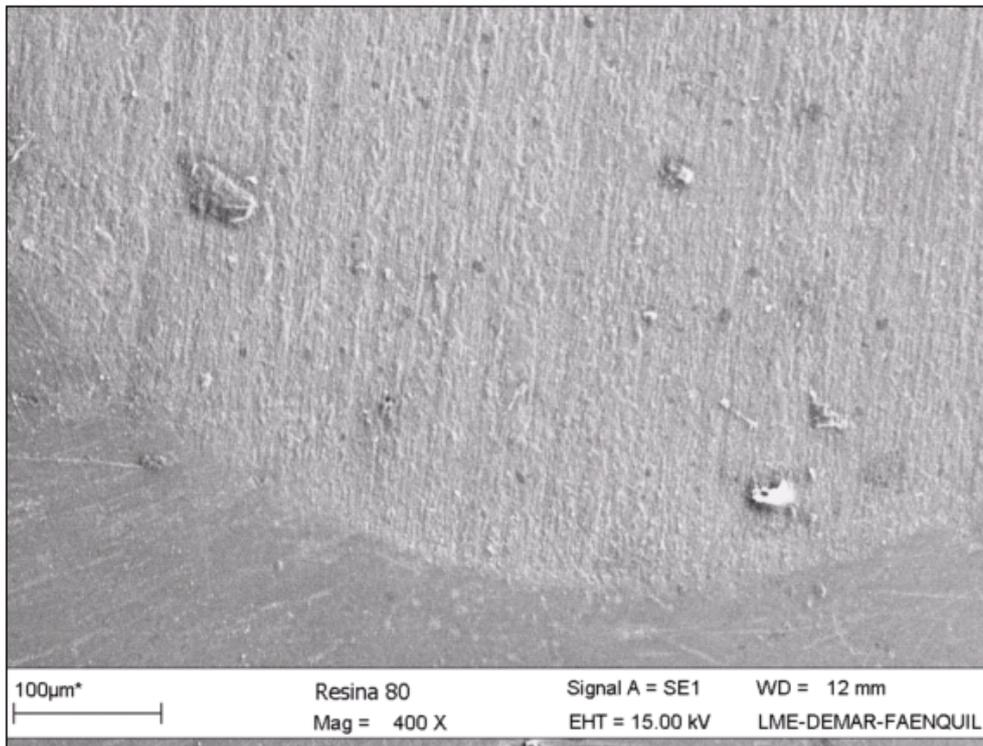
Illustration 5. Photo of the border of the crater obtained in the *Test of micro Abrasion Ball Cratering* test, SEM, resin F
