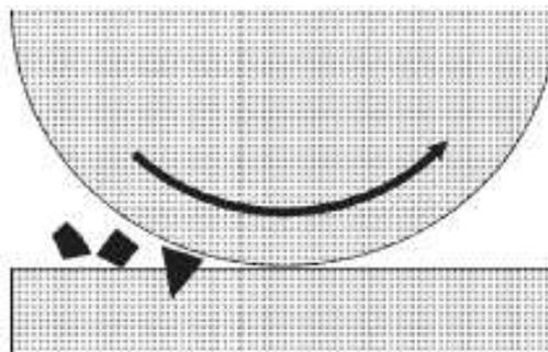
Illustration 1 depicts the mechanism of wear of an angular particle.
