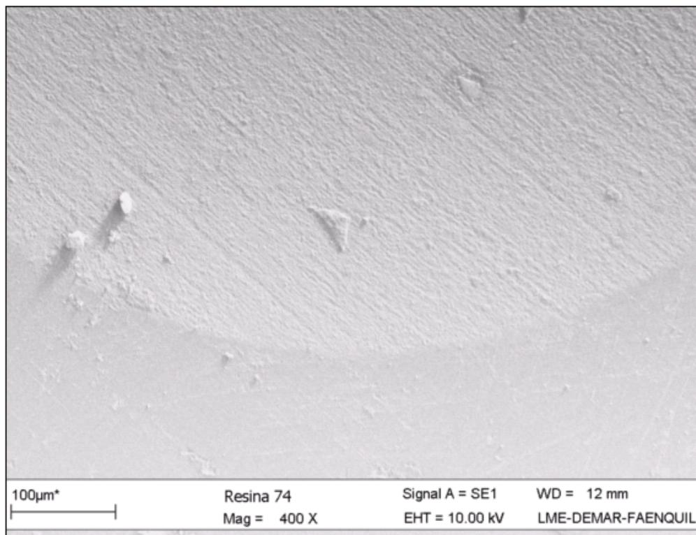
Illustration 4 . Photo of the border of the crater obtained in the *Test of micro Abrasion Ball Cratering*, SEM, resin B
