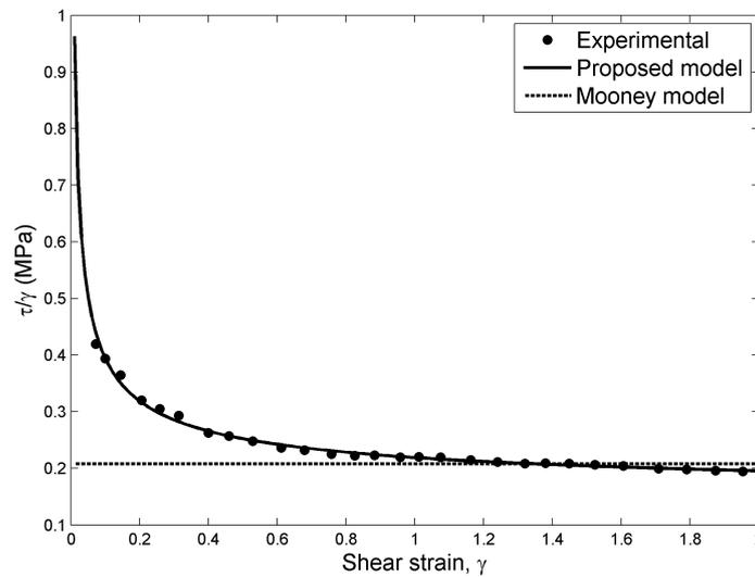
Figure 7. Shear stress divided by shear strain vs. shear strain.
