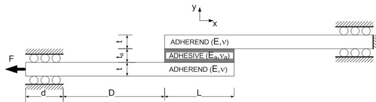
Figure 2. Schematic of simple shear deformation
