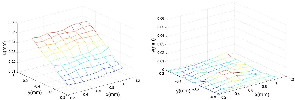
Figure 4. Full-field displacements  $u(x,y)$  and  $v(x,y)$  for applied load equal to 50 N.
