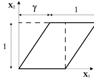
Figure 1. Schematic of simple shear deformation
