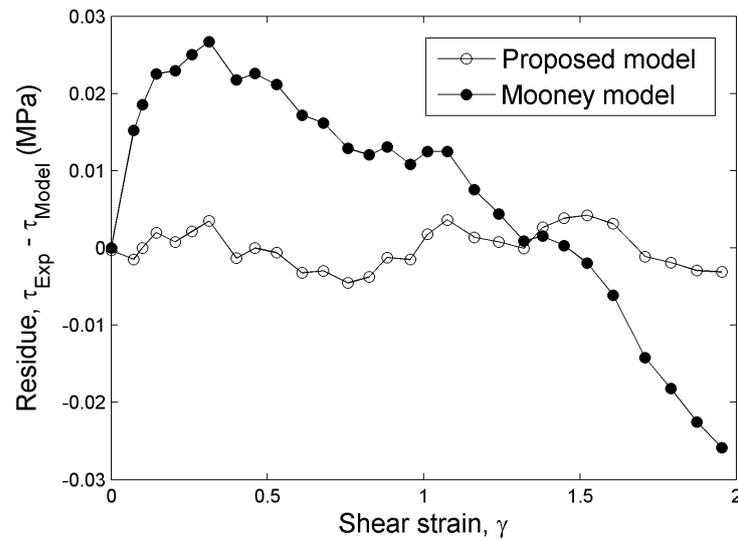
Figure 8. Residue,  $\tau_{Exp} - \tau_{Model}$ , for different shear strain: comparison between Mooney and proposed model
