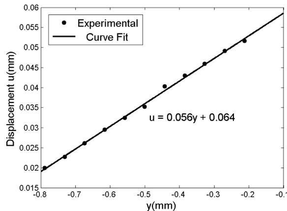
Figure 5. Average value of displacement  $u(x,y)$  along direction  $x$  as a function of  $y$  for applied load equal to 50 N.
