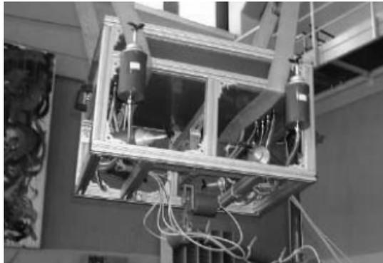
Figure 8. Underwater vehicle Prototype (Bessa *et al.*, 2008)
