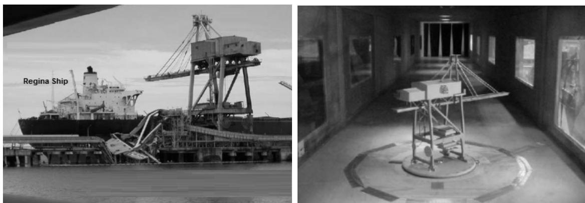
Figure 9. Structural Accident of a ship unloader and prototype (Batista *et al.*, 2005).
