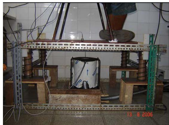
**Figure 2: Photo of the setup used for the WBV Reading Tests**
