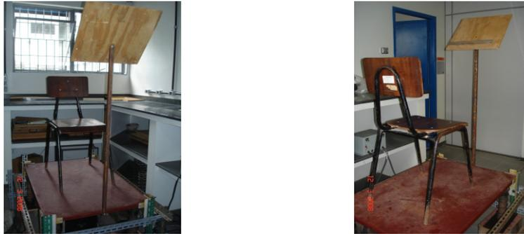
**Figure 3: Details of the pedestal and chair used during the reading WBV tests**
