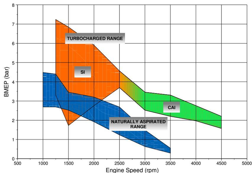
Figure 2 Comparison between NA and Turbocharged CAI ranges
