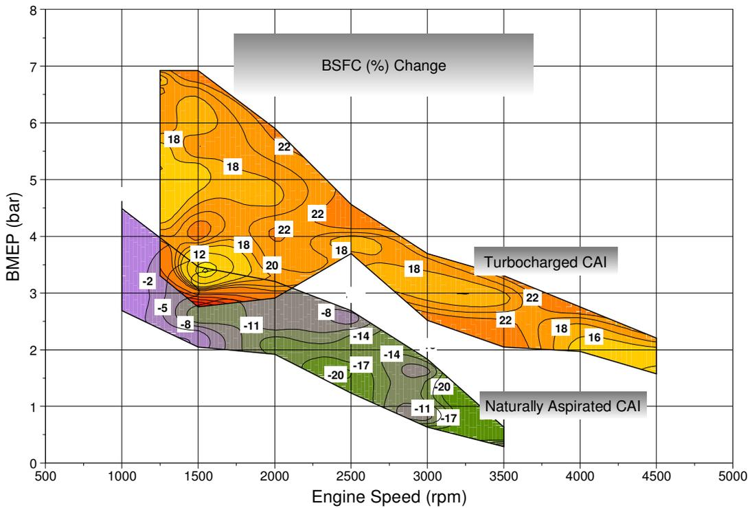
**Figure 7 Change in BSFC (%) of the NA and Turbocharger CAI engine over a standard SI engine**
