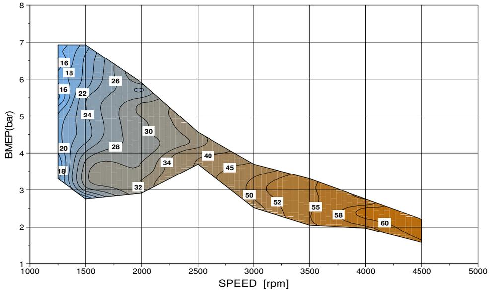
**Figure 3 Exhaust residual concentration as a function of speed and load (%)**
