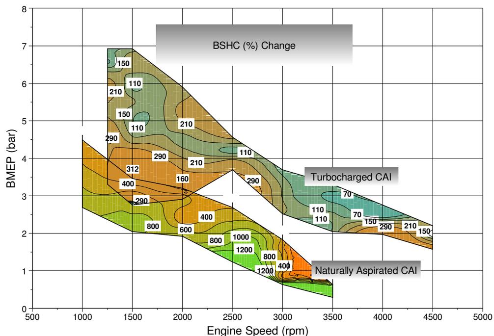
**Figure 5 Change in BSHC (%) of the NA and the Turbocharged CAI engine over a standard SI engine**
