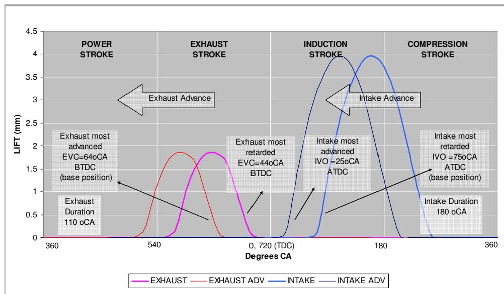
Figure 1 Intake and Exhaust cam profiles and VCT range for the turbocharged operation
