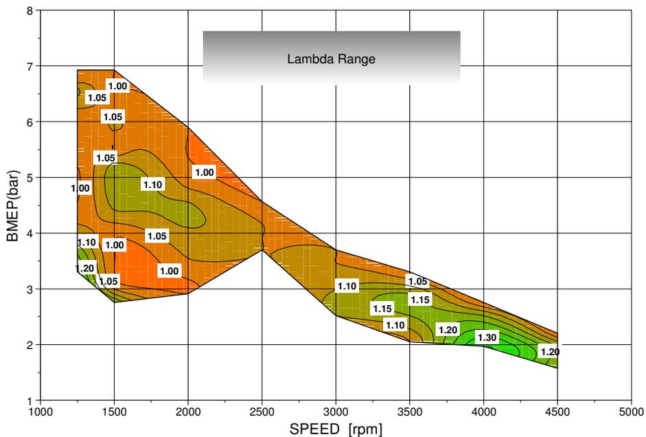
**Figure 4 Lambda range for the turbocharged operation for minimum BSFC**
