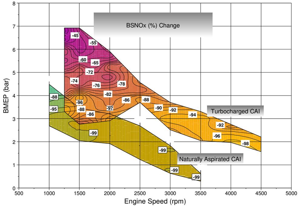
**Figure 6 Change in BSNOx (%) of the NA and the Turbocharged CAI engine over a standard SI engine**
