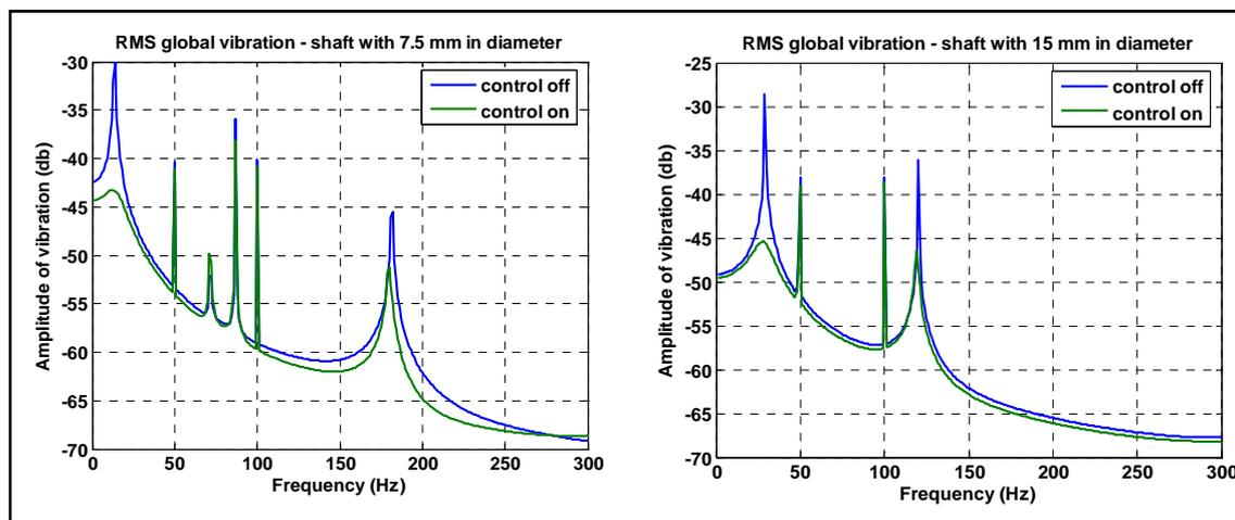
**Figure 4. RMS global vibration with and without active control (cases B and E)**
