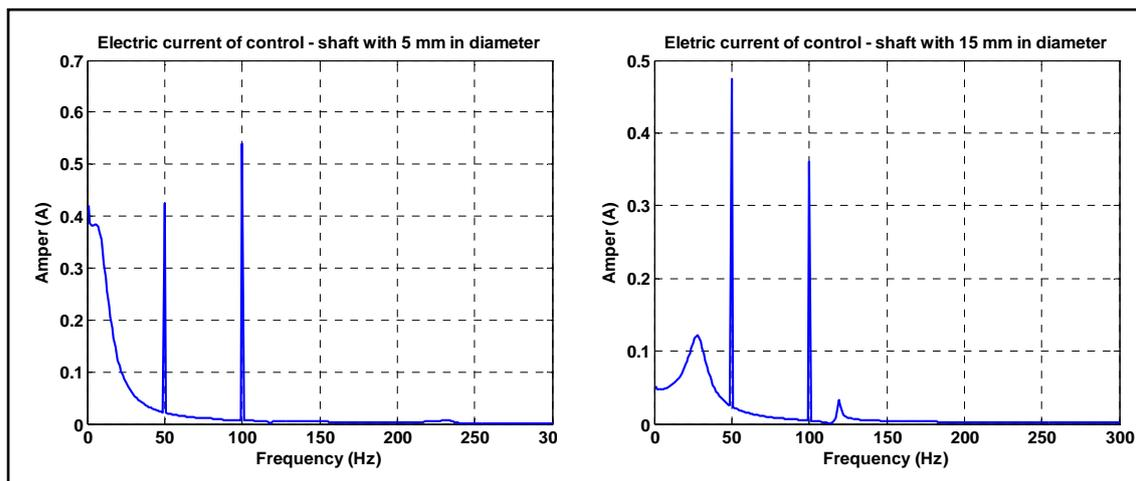
Figure 8. Electric current of control – shaft with 5mm and 15 mm in diameter
