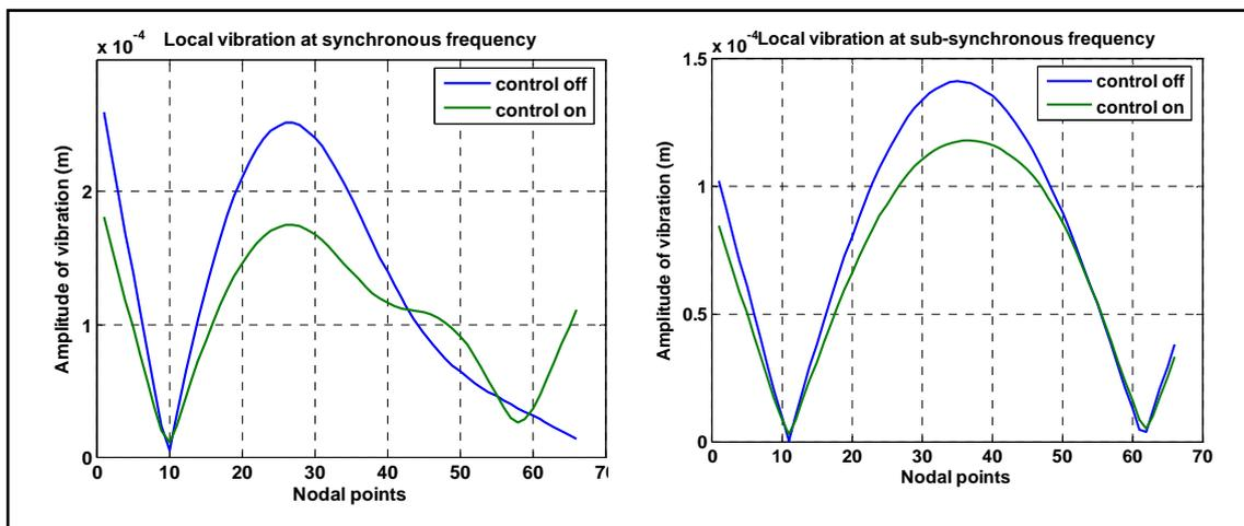
Figure 5. Vibration along of rotor before and after control - shaft with 5 mm in diameter (case A)
