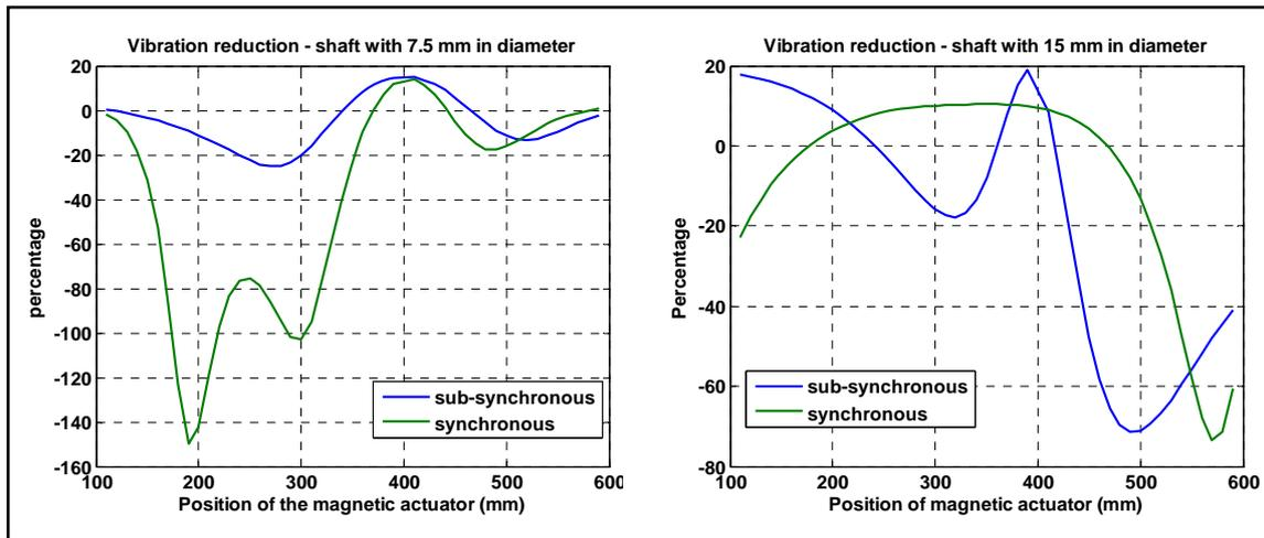
**Figure 3. RMS vibration reduction as a function of actuator position along of the rotor (cases B and E)**
