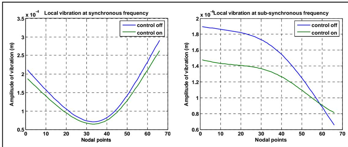
Figure 7. Vibration along of rotor before and after control - shaft with 15 mm in diameter (case E)
