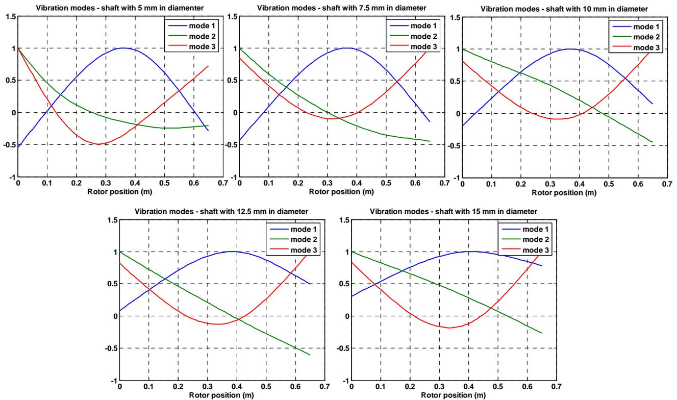
Figure 2. Mode shapes as a function of the rotor flexibility
