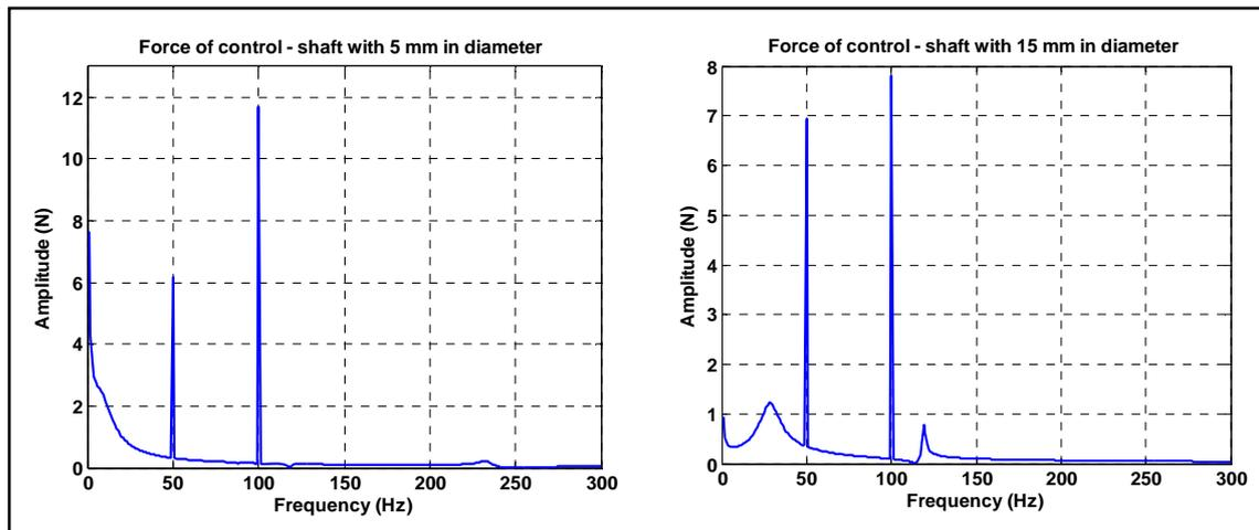
Figure 9. Force of control – shaft with 5 mm and 15 mm in diameter
