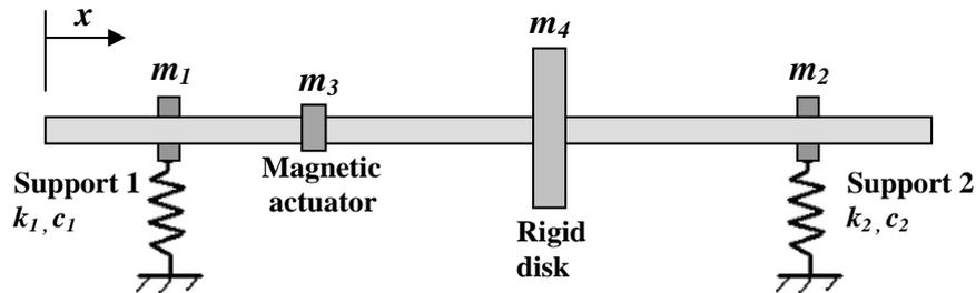
**Figure 1. Sketch of rotor for analysis of active control of vibration with magnetic actuator****Table 2. Properties of the conventional bearings**
