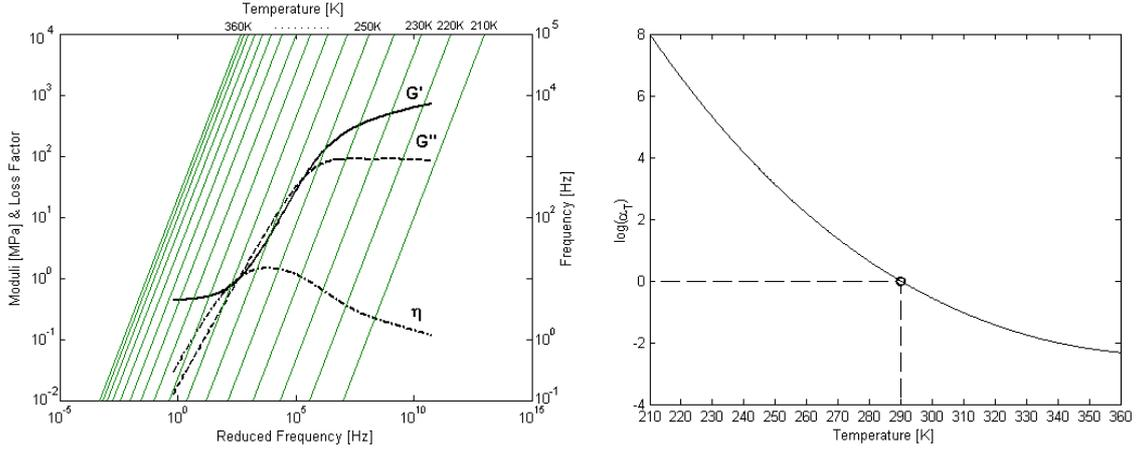
Figure 4. Master and shift factor curves for the 3M™MSD112 viscoelastic material.
