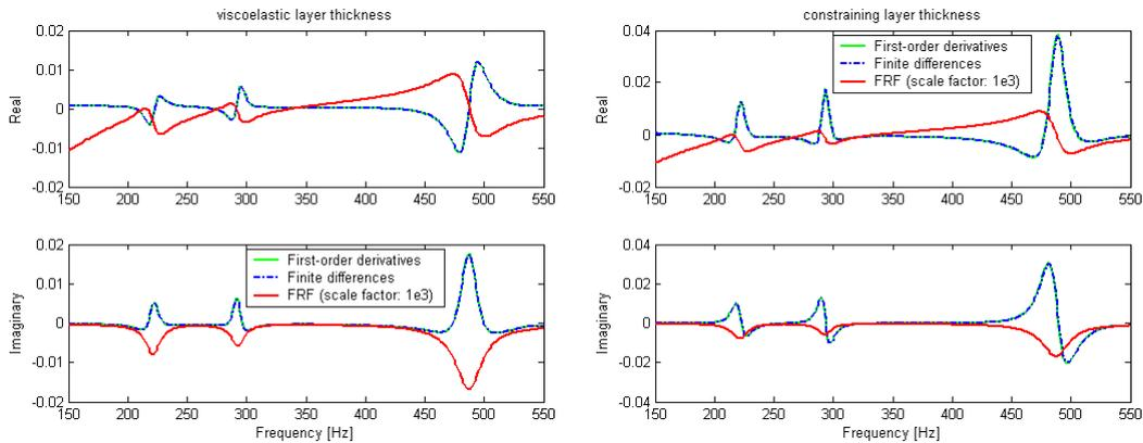
Figure 5. FRF sensitivities with respect to the thicknesses of the viscoelastic and constraining layers.
