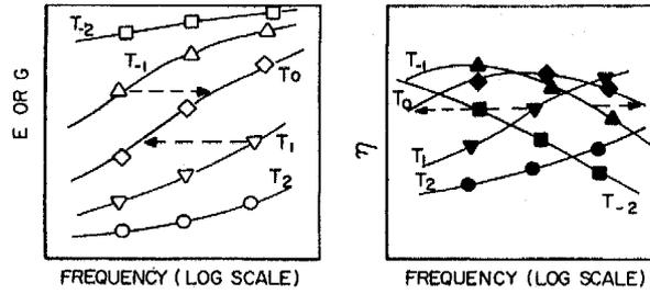
Figure 1. Illustration of the Frequency-Temperature Superposition Principle (adapted from Nashif *et al.* (1985)).
