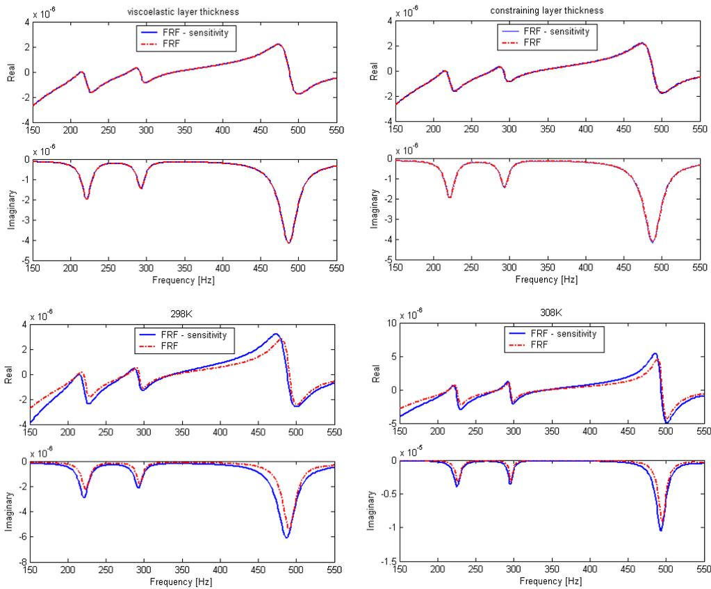
Figure 7 – Exact and first-order approximations of the FRFs of the system perturbed by variations of the design variables
