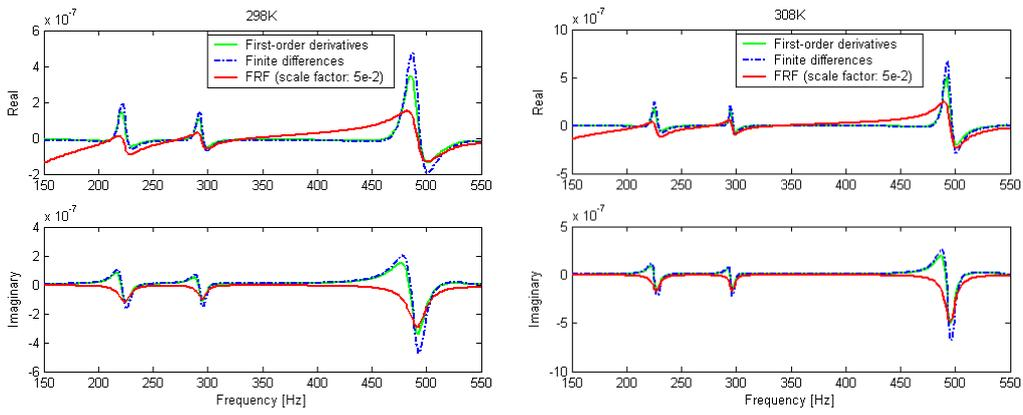
Figure 6. Sensitivities of the FRF with respect to temperatures for nominal temperature values 298K and 308K.
