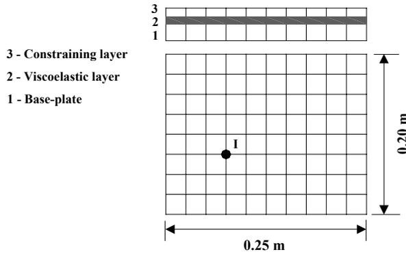
Figure 3. Illustration of the FE model of a free plate with full surface treatment.
