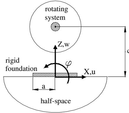
Figure 3: modelling of a rigid foundation for machine supporting
