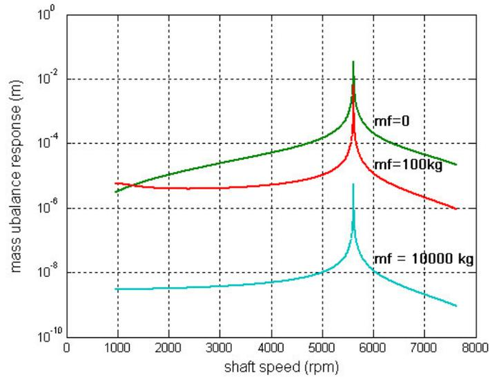
Figure 10: Influence of the foundation mass in dynamic response of rotating machinery
