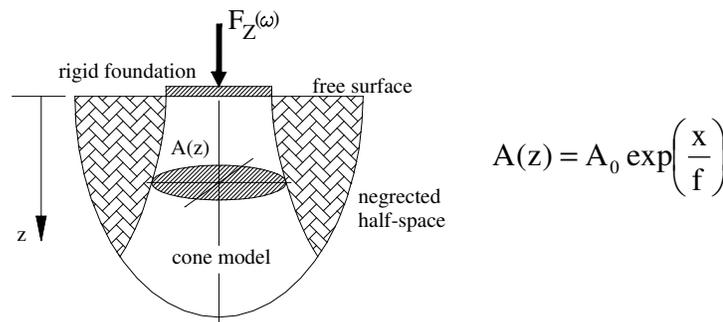
Figure 4: model of exponential cone for  $N_{wz}(\omega)$
