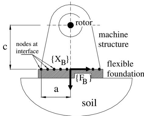
Figure 2: supporting system of a flexible foundation
