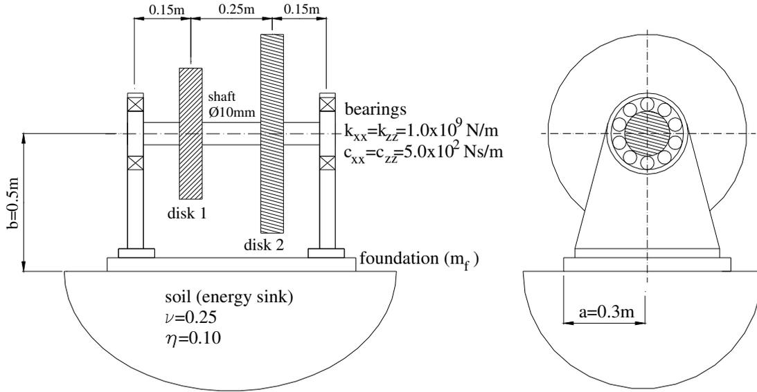
Figure 9: Geometry of the rotating machinery
