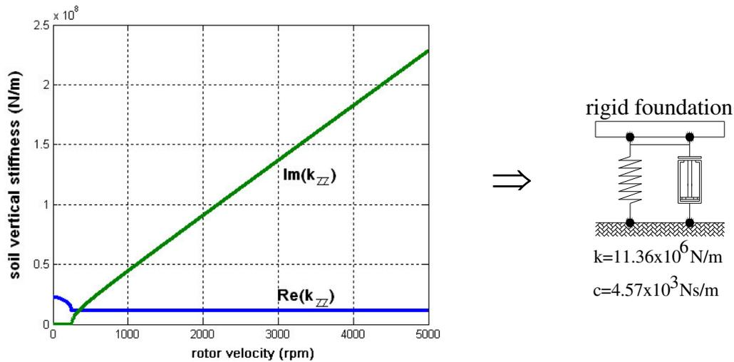
Figure 5: behaviour of  $k_{wz}(\omega)$  for an exponential cone model
