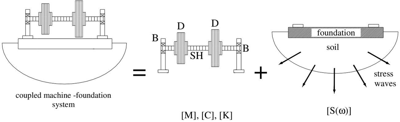
Figure 1: decomposition of the original coupled system into machine and support sub-systems
