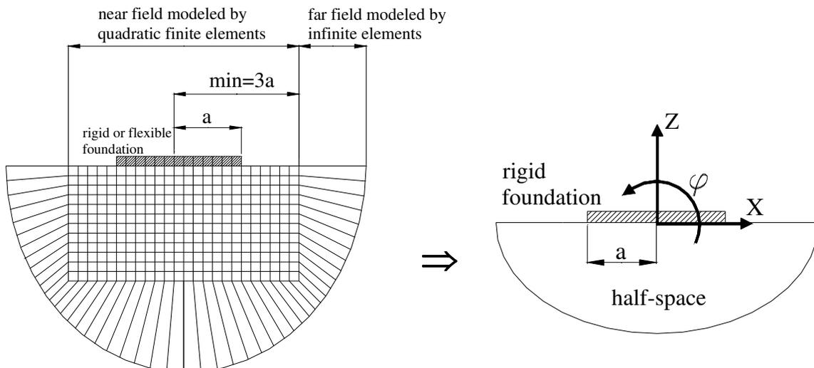
Figure 6: Modelling technique of a homogeneous half-space by a hybrid finite/infinite element mesh
