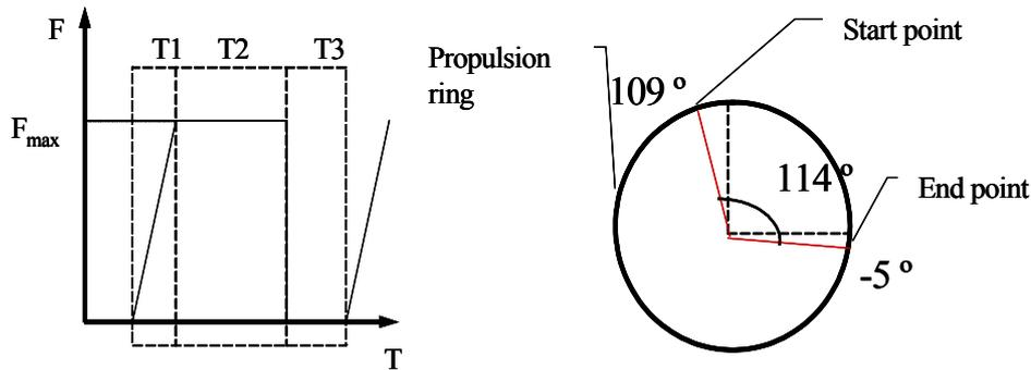
Figure 1. Characterizes of Propulsion Force definition
