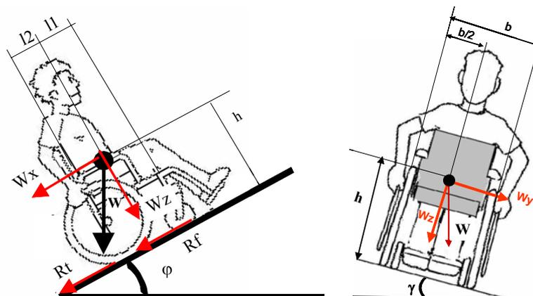
Figure 4. Forces diagram acting over the system in double inclination plane
