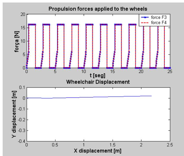
Figure 9. Wheelchair displacement with different propulsion forces acting over a system with servo assisted mechanism
