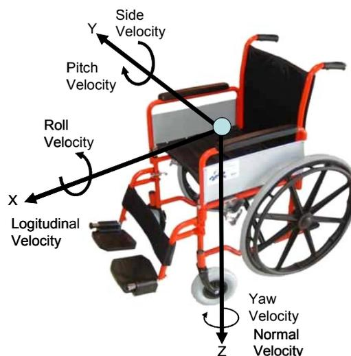
Figure 2. Definition of the Reference System according to SAE
