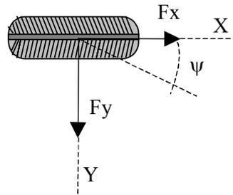
Figure 3. Forces scheme actuating over the wheel
