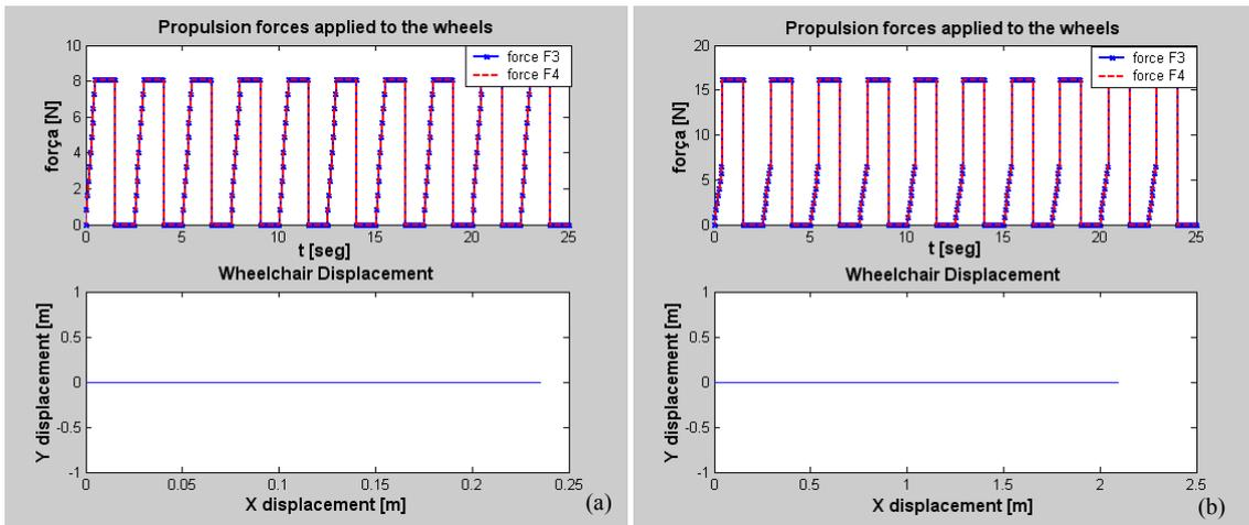
Figure 8. Comparison between a system without servo assisted mechanism (a) and a system with a servo assisted mechanism (b)
