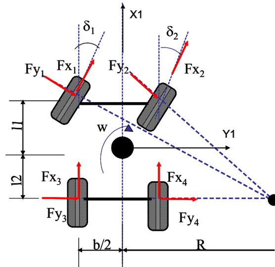
Figure 5. Free Body Diagram for the wheelchair
