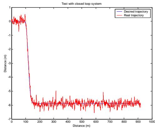
**Figure 8. Test with noise at the measurement of state variable - SNR =  $-3\text{dB}$**
