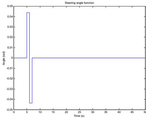
**Figure 3. Input function for the frontal steering angle**
