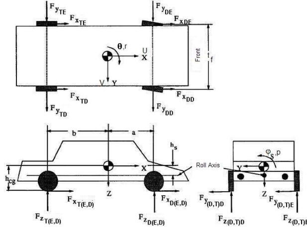
**Figure 1. Distribution of forces and moments in a ground vehicle**
