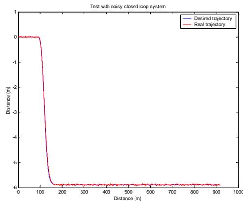
**Figure 9. Test with noise at the controller output - SNR =  $-4\text{dB}$**
