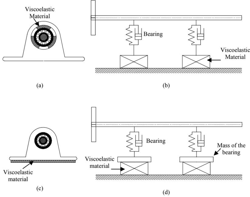
Figure 2. Model of bearings with viscoelastic material.
