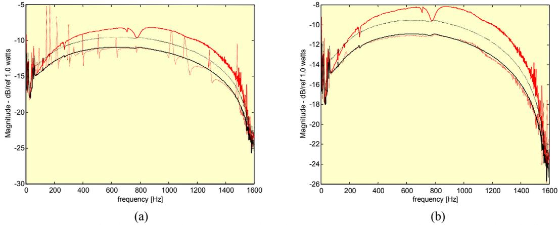
Figure 6: Power terms for the BEAM with:(a) LIGHT damping and (b) HEAVY damping; source with periodic CHIRP signal: ---  $|\bar{Q}|$  input power, —  $|MAP|$ , —  $|MP|$ , ---  $|CP|$
