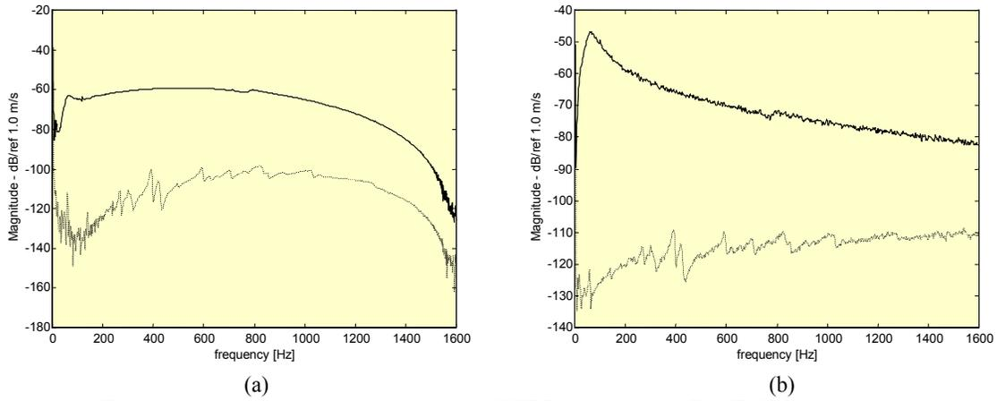
Figure 3: Source velocity with:(a) periodic CHIRP signal and (b) RANDOM signal under:
