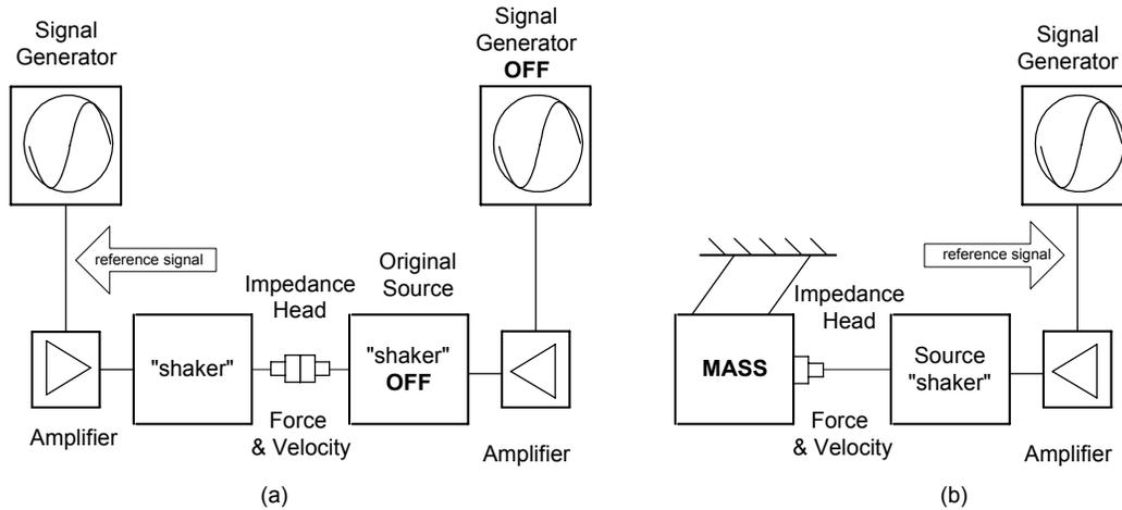
Figure 8: Experimental Setup of Source Mobility: (a) “direct method”; (b) “mass method”
