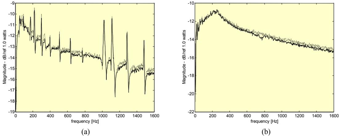
Figure 5: Power input into the BEAM with: (a) LIGHT damping and (b) HEAVY damping; source with RANDOM signal:  $-\overline{|Q|}$  Eq. (4),  $--- \overline{|Pin|}$  Eq. (1).
