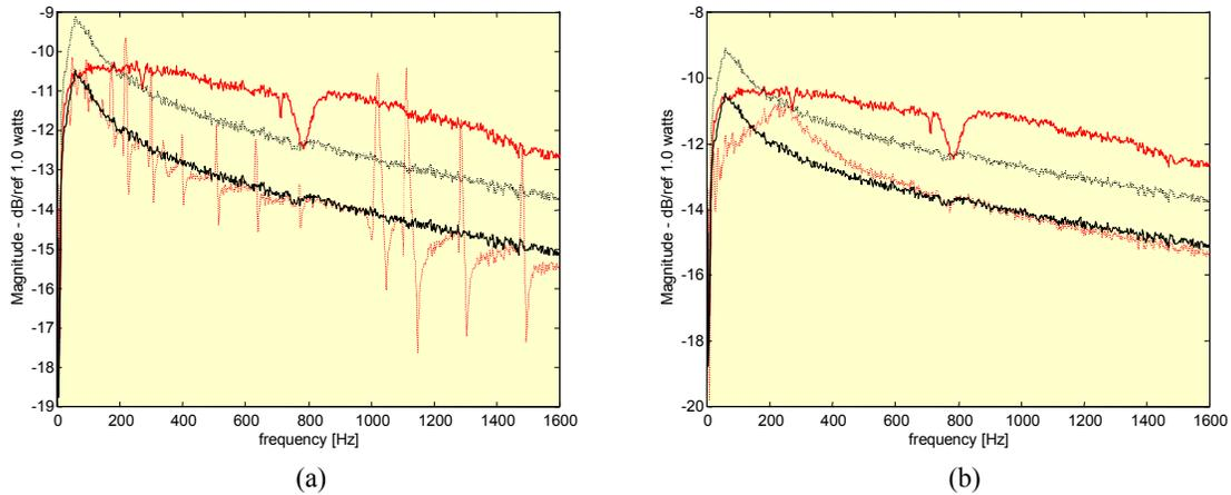
Figure 7: Power terms for the BEAM with:(a) LIGHT damping and (b) HEAVY damping; source with RANDOM signal: ---  $|\bar{Q}|$  input power, —  $|MAP|$ , —  $|MP|$ , ---  $|CP|$
