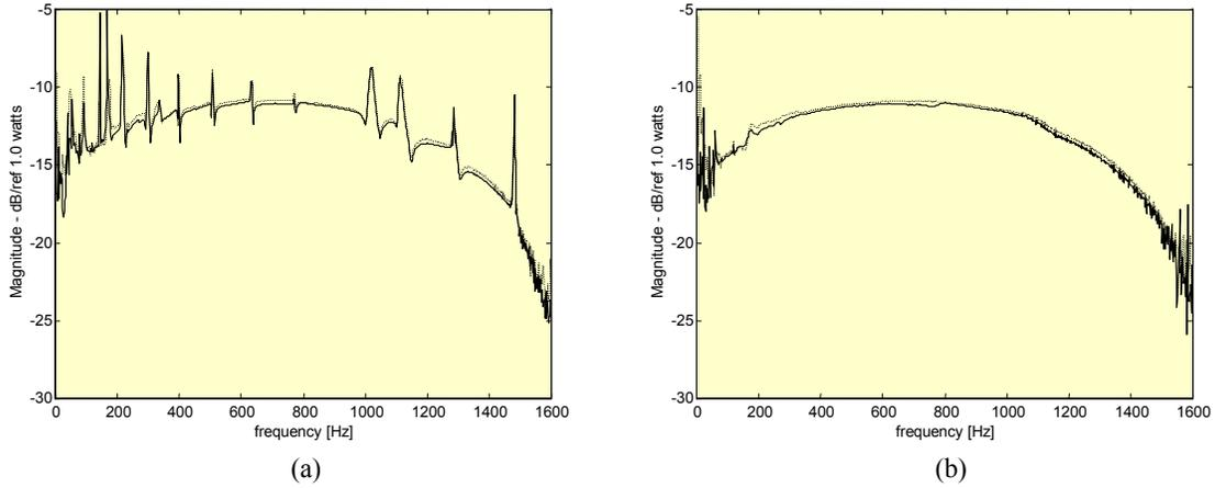
Figure 4: Power input into the BEAM with: (a) LIGHT damping and (b) HEAVY damping; source with periodic CHIRP signal:  $-\overline{|Q|}$  Eq. (4),  $--- \overline{|Pin|}$  Eq. (1).
