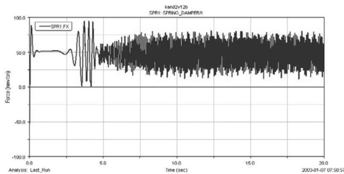
Figure 17. Rod suspension spring force.
