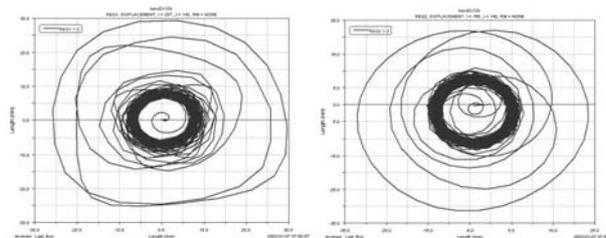
Figure 13. Upper orbit and Lower orbit.
