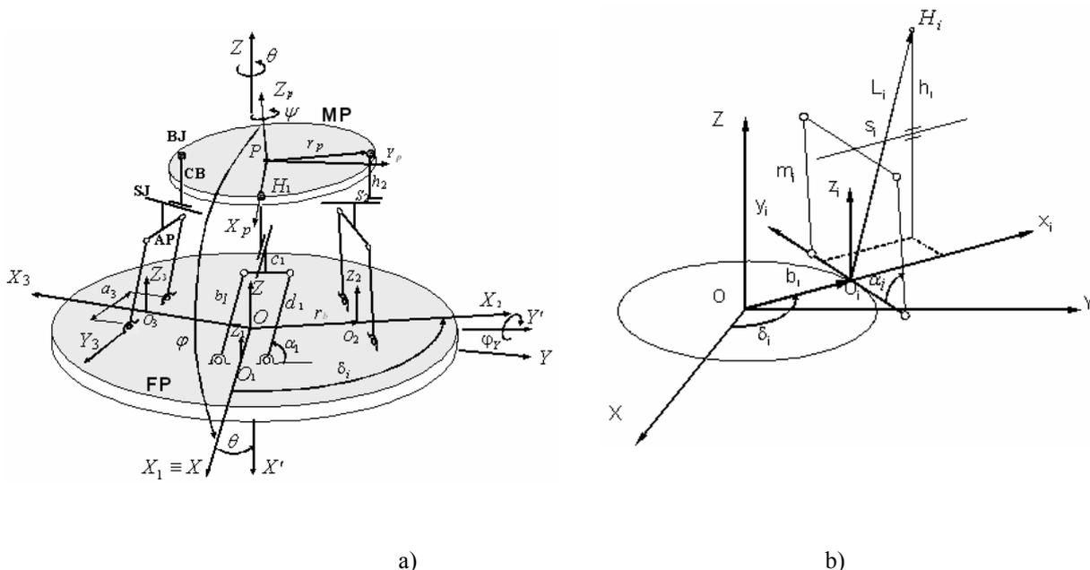
Figure 1. a) Kinematic chain of CaPaMan. b) Parameters associated to the  $i$ -th leg.
