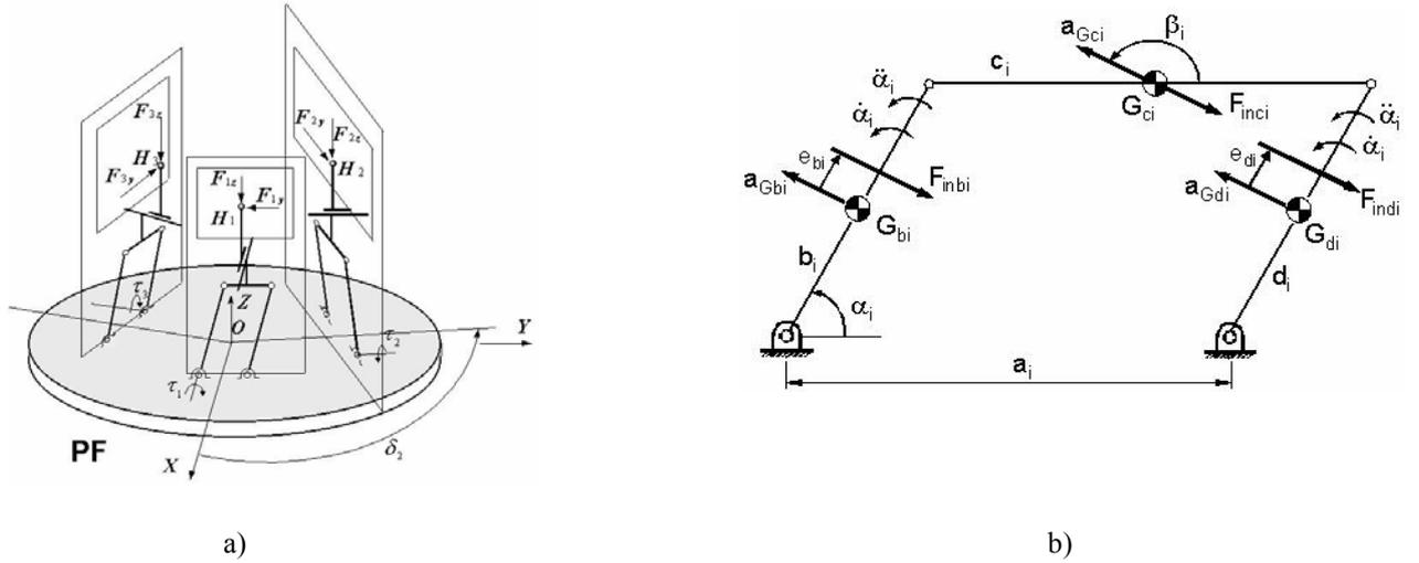
Figure 2. a) Forces acting at the spherical joints. b) Forces in the  $i$ -th articulated parallelogram ( $i=1,2,3$ ).
