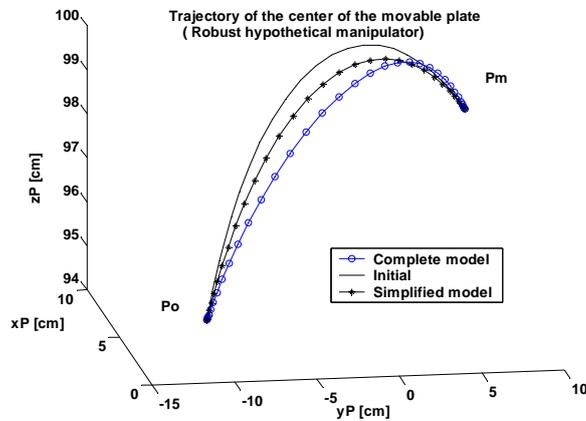
Figure 6- A 3D plot of the position of the center of the movable plate for Robust Hypothetical Manipulator.
