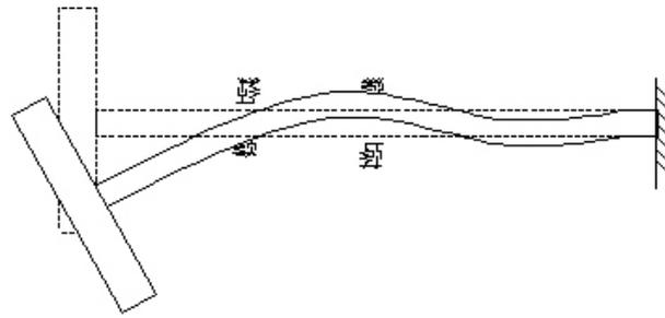
Figura 9 – Shape of the shaft under operation condition
