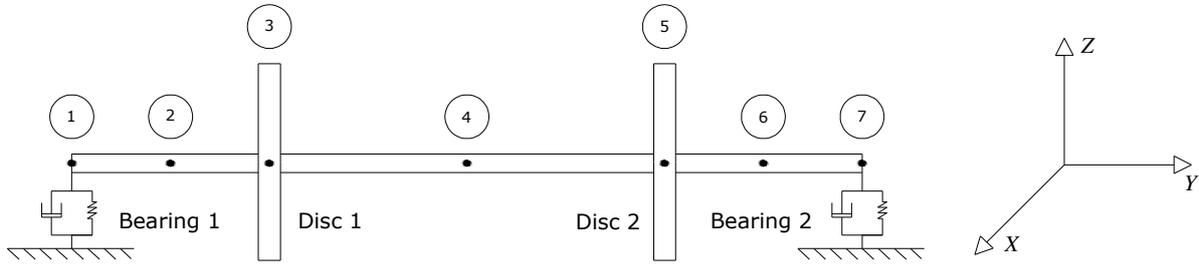
Figure 2 – FEM rotor model.
