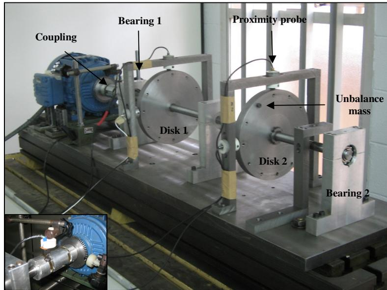
Figure 3 – Experimental test rig.
