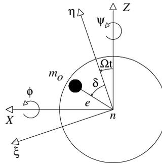
Figure 1 – Node  $n$  of the rotor disk with unbalance.
