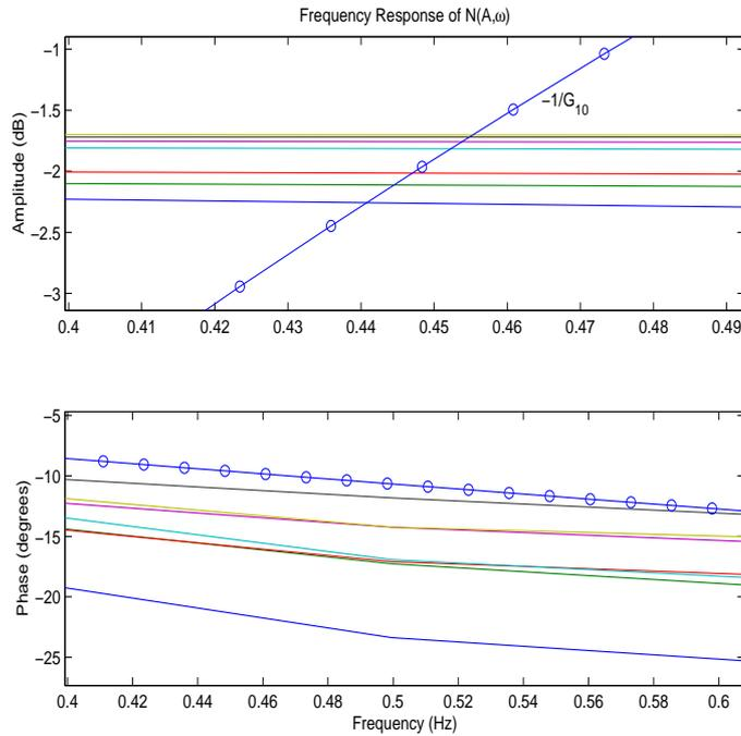
Figure 7 – Frequency response of the nonlinear hydraulic actuator and the inverse of the  $G_{10}$  system.
