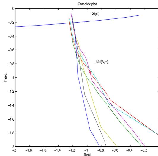
**Figure 5 – Nyquist plot of the linear element and the inverse of the nonlinear element. It is possible predict a limit-cycle in a closed loop with both elements.**
