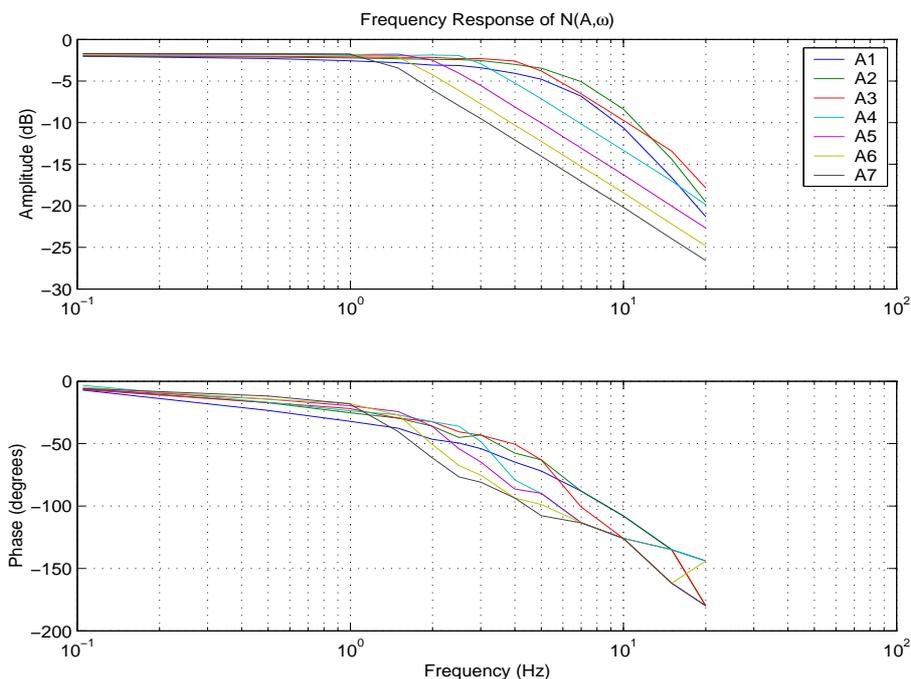
**Figure 2 – Frequency response of the hydraulic actuator. Each curve represents one amplitude for the sinusoidal input.**
