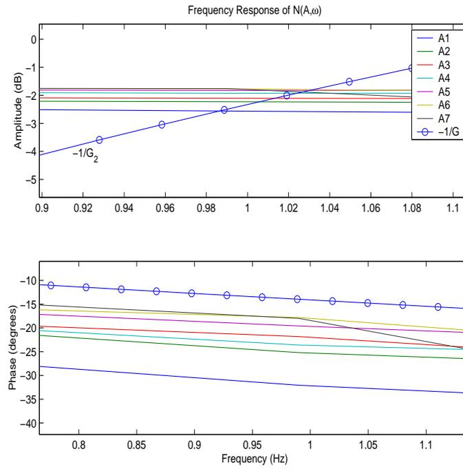
Figure 6 – Frequency response of the nonlinear hydraulic actuator and the inverse of the  $G_2$  system.
