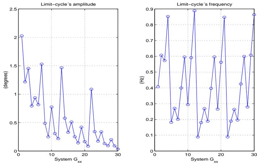
Figure 3 – Frequency and amplitude of the limit cycle for each closed loop experiment.
