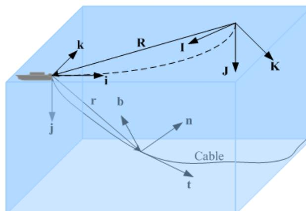
Figure 2 - Reference System: Inertial -  $(\mathbf{I}, \mathbf{J}, \mathbf{K})$ ; Vessel  $(\mathbf{i}, \mathbf{j}, \mathbf{k})$ ; Local  $(\mathbf{t}, \mathbf{n}, \mathbf{b})$
