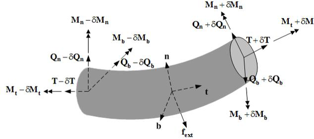
**Figure 3 – Forces and Moments in a Element of Cable with Length  $\delta p$**
