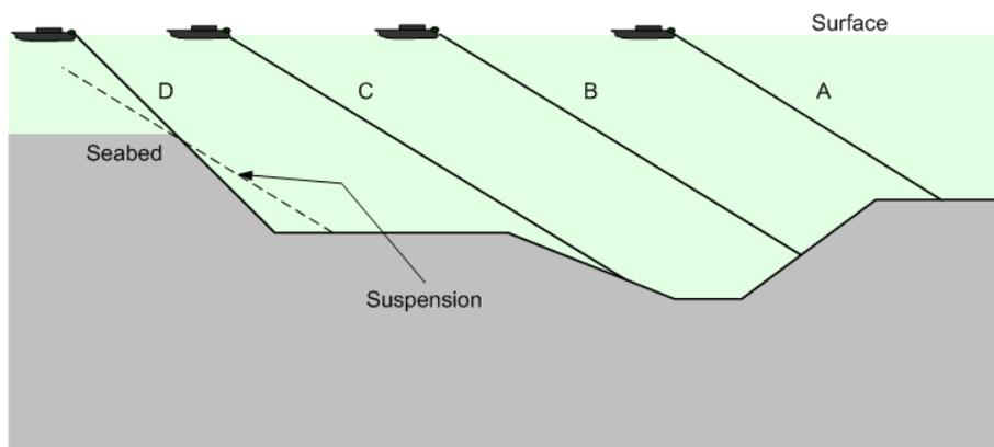
Figure 1 – Sketch for laying in a irregular seabed: A- horizontal seabed; B- Descending Seabed; C – Ascending Seabed with slope lower than the cable inclination; D – Descending Seabed with slope greater than the cable inclination
