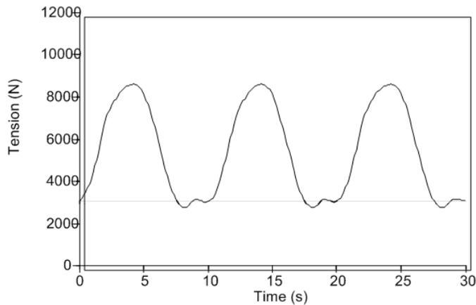
Figure 5 – Top tension for a wave simulation of a light armoured cable
