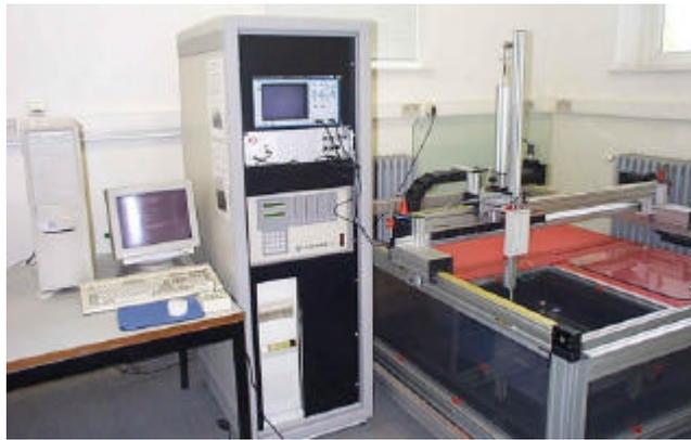
Figure 6 – Ultrasonic C-Scan equipment at LCPC of Katholieke Universiteit Leuven (Belgium)
