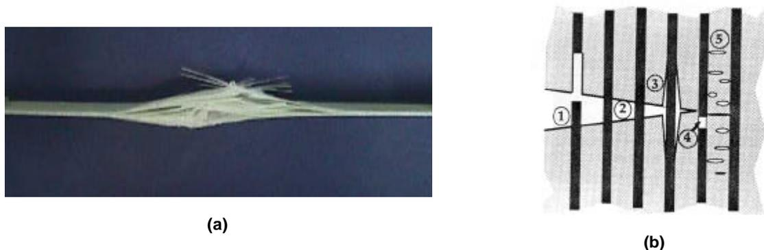
**Figure 1 – (a) Composite failure mechanics: intra-ply and inter-ply failures;(b) Intra-ply damages(Anderson, 1995)**
