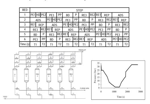
Figure 1 - Sequence of steps and pressure variation of a bed on a complete PSA cycle.
