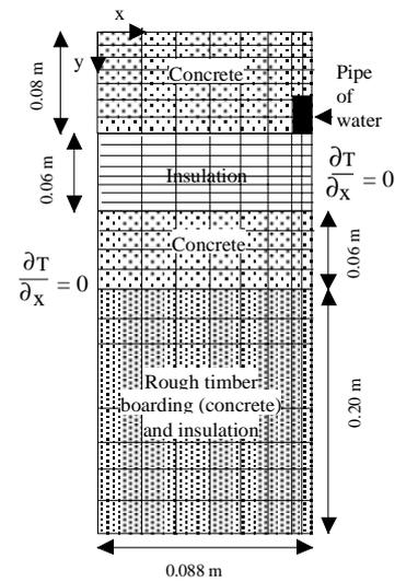
Figure 3- Elementary frame of the heating floor
