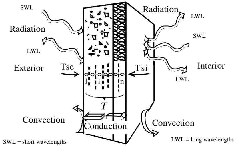
Figure 1- Control volumes for an elementary component of the envelope and boundary conditions
