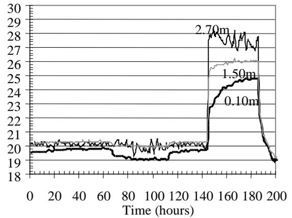
Figure 9- EC : Mesured air temperature  $T_a$  at different level of the cell (°C)
