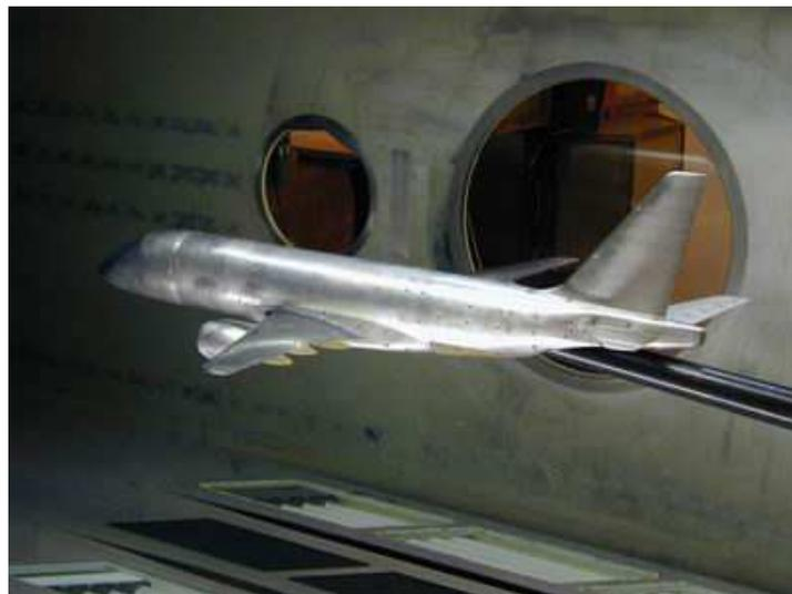
Figure 10. Transonic pressurized tunnel test - EMBRAER 170 at DNW/HST.
