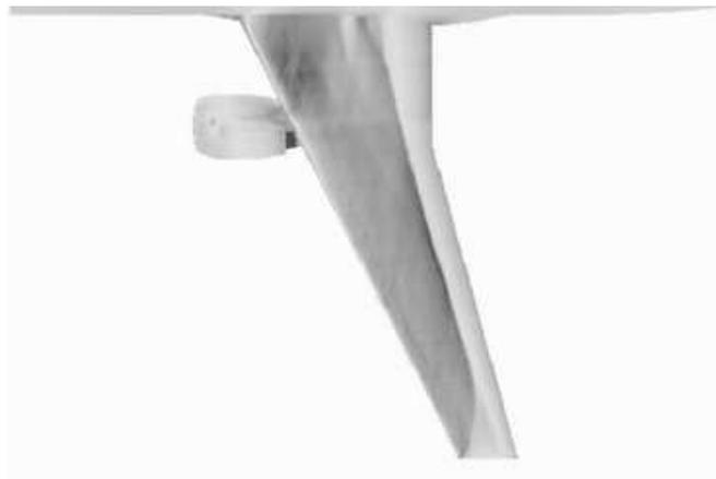
Figure 5b. CFD pressure distribution results for wing-pylon-nacelle configuration (EMBRAER 170)
