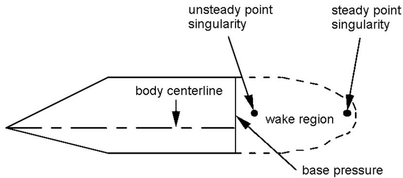
Figure 4. Singularities placed behind a body to represent its wake in ZAERO (adapted from Zona Technology (2003b)).
