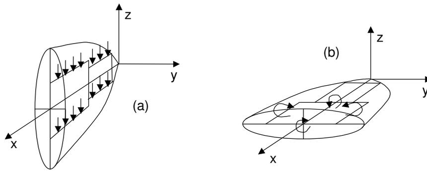
Figure 2. Doublet lines (a) and quadrilateral vortex (b) used to model slender bodies in MSC/NASTRAN (adapted from Giesing et al. (1972)).
