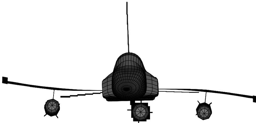
Figure 14. Representation of the flutter mode.
