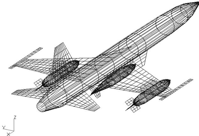
Figure 8. Lifting surface and slender body elements used in the model with bodies and fins in MSC/NASTRAN.
