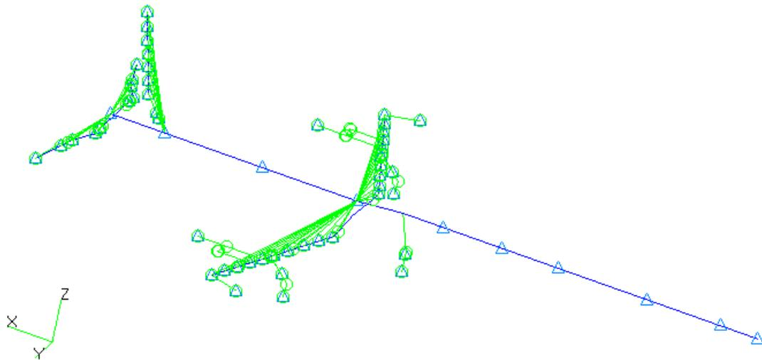
Figure 5. Simplified dynamic-structural model of the aircraft with external stores used for flutter analysis.
