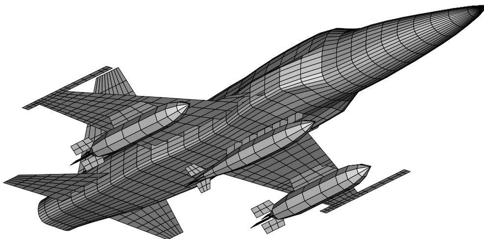
Figure 6. Aircraft surface discretizations for aerodynamic model with bodies and fins used in ZAERO.
