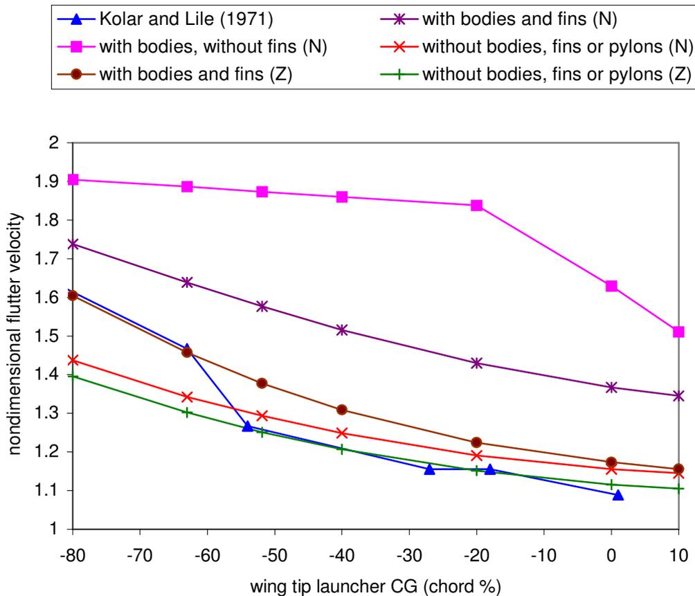
Figure 10. Flutter velocity dependence on the position of the tip launcher CG.
