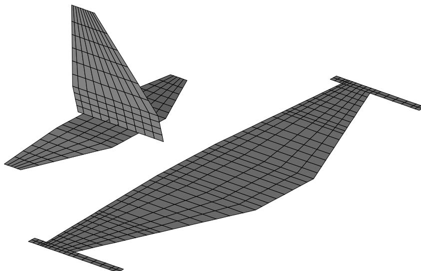
Figure 7. Lifting surfaces discretization used in MSC/NASTRAN and in ZAERO for the model without bodies or fins.
