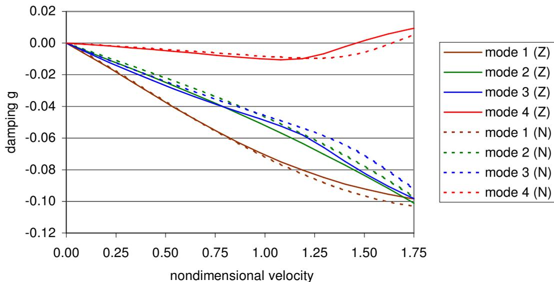
Figure 11. Damping curves obtained with the models with external stores and fins.
