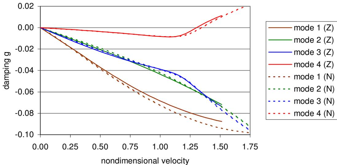
Figure 13. Damping curves obtained for the models without external stores or fins.
