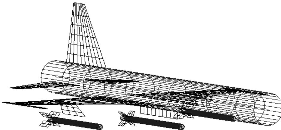
Figure 9. Lifting surface and interference elements used in the model with bodies and fins in MSC/NASTRAN.
