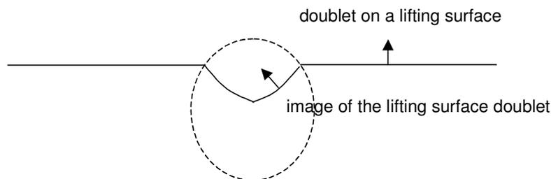
Figure 1. Image of lifting surfaces inside an interference tube (represented by the dashed line) of elliptical cross section. (adapted from Giesing at al. (1971)).
