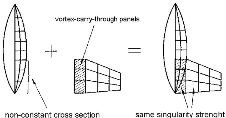
Figure 3. Doublet panels placed inside a body, to avoid a lifting surface root vortex in ZAERO (adapted from Zona Technology (2003b)).
