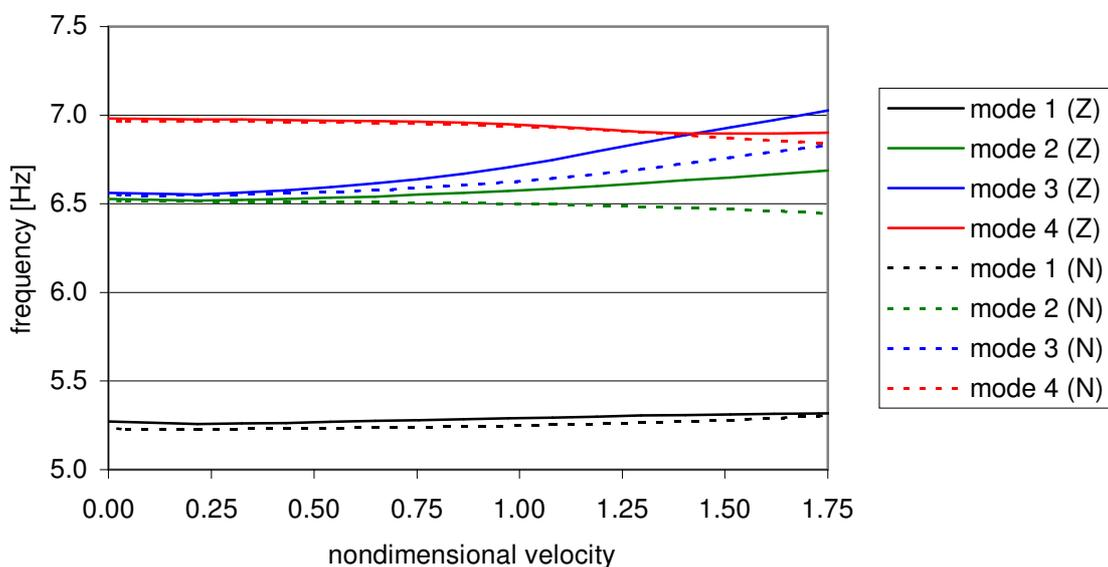
Figure 12. Frequency curves obtained with the models with external stores and fins.
