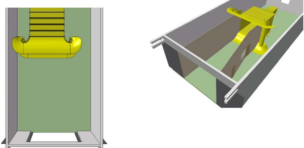
Figure 11. Comparison of the original tunnel intake, at left, with the new inlet chamber at right
