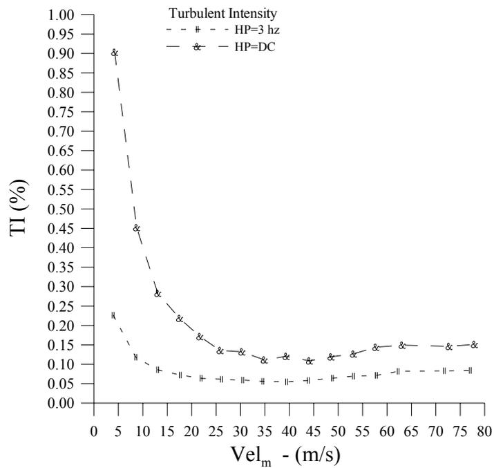
Figure 12. Influence of the filter on the turbulence intensity for different velocities at the test section
