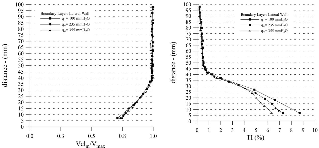
Figure 7. Velocity profiles and turbulence intensity at the tunnel lateral wall for three different fan rotations.
