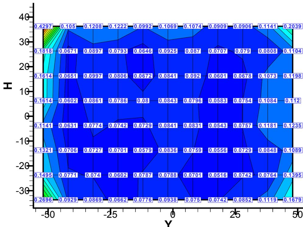
Figure 13. Turbulence intensity at the test section with new inlet chamber
