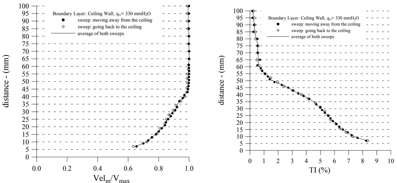
Figure 9. Velocity profiles and turbulence intensity at the tunnel ceiling for 800 rpm.
