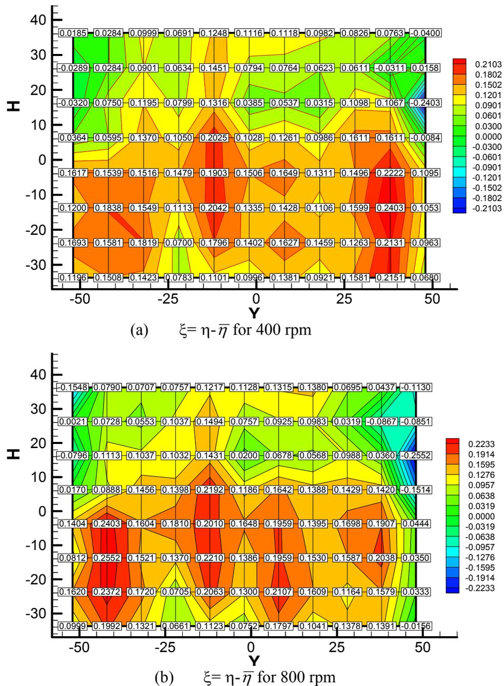
Figure 5. Flow uniformity distribution at a cross-plane located at the test section mid length.
