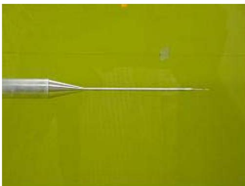
Figure 10. Hot-wire anemometer probe inside the test section.
