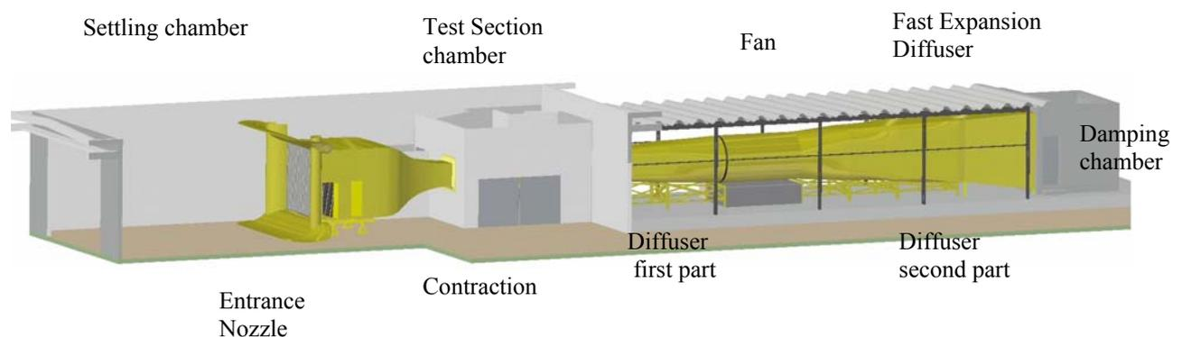
Figure 1. View of ITA's low-speed wind tunnel inside Prof. Feng Aeronautical Engineering Laboratory.
