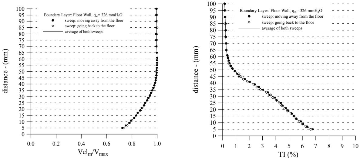
Figure 8. Velocity profiles and turbulence intensity at the tunnel floor for 800 rpm.
