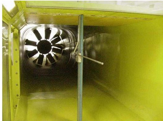
Figure 3. Pitot-static tube mounted within the test section.
