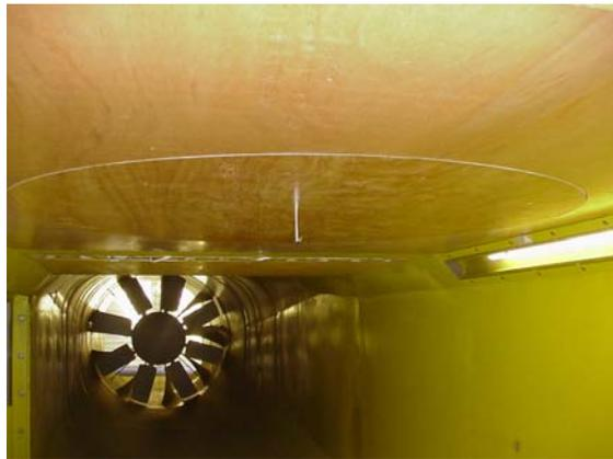
Figure 6. Hot-wire anemometer mounted at the test section
