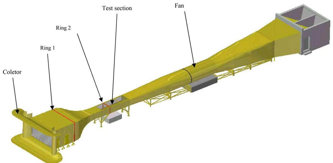
Figure 4. Tunnel rings locations
