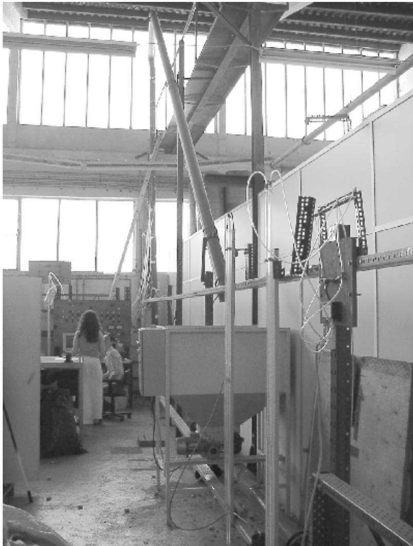
Figure 2. Image of the experimental installation. In the first plan it can be seen the orifice plate air flow meter and the corks feeding hopper.
