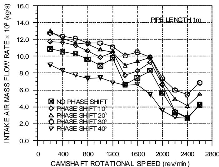
Figure 4 – Variation of the intake air mass flow rate with intake valves phase shift and camshaft rotational speed for the intake pipe length of 1.0 m.
