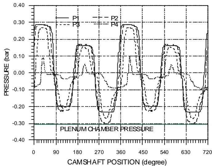
Figure 6 – Pressure along the intake conduit during an engine cycle at the camshaft speed of 1200 rev/min without intake valves phase shift.
