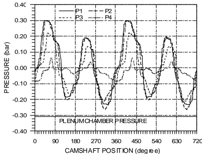
Figure 7 – Pressure along the intake conduit during an engine cycle at the camshaft speed of 1200 rev/min and intake valves phase shift angle 40 camshaft degrees.
