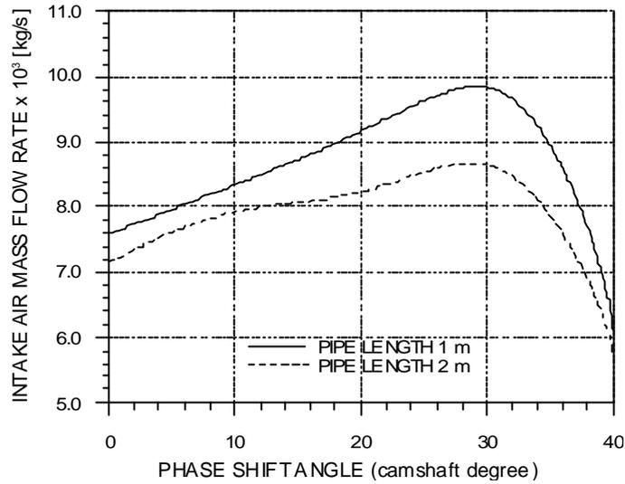
Figure 5 – Variation of the average mass flow rate in the speed range tested with intake valve phase shift angles for the intake conduits of 1.0 m and 2.0 m.
