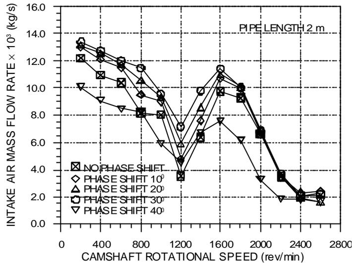
Figure 3 – Variation of the intake air mass flow rate with intake valves phase shift and camshaft rotational speed for the intake pipe length of 2.0 m.
