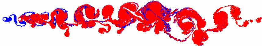
Figure 2. Position of the binary-vortex street at  $t=75$  for the spacing gap  $g/d=4.5$ .
