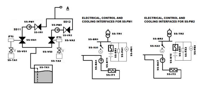
Figure 1. Illustrative Technological Safety System SS
