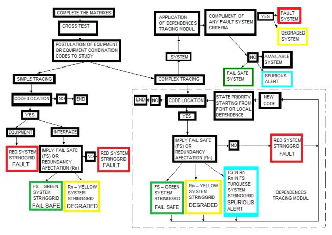
Figure 2. Tracing Algorithm implemented in the computer code SECURE A-Z
