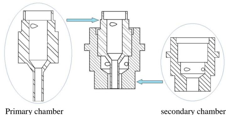
Figure 4. Scheme of the dual centrifugal injector.
