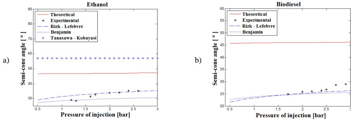
Figure 8. Cone angle generated in the primary chamber of the injector to a) hydrated ethanol; b) soy biodiesel.
