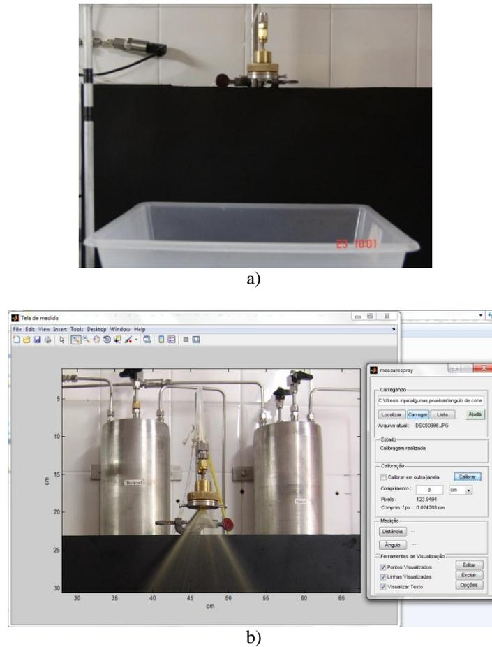
Figure 6. a) Experimental setup and b) GUI for image processing.
