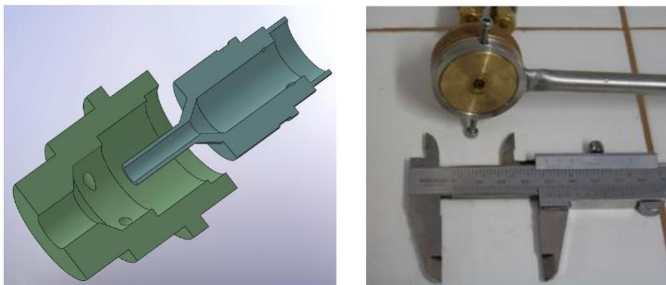
Figure 5. Cut view and photo of the injector.
