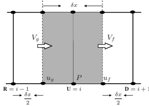
Figure 1. Sketch of upwind-biased stencil at point  $P$
