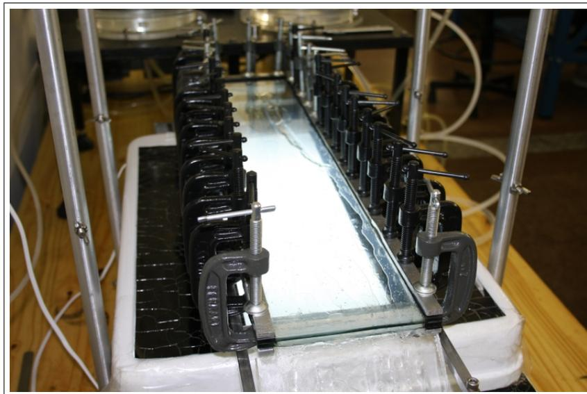
Figure 4. The Hele-Shaw cell apparatus.
