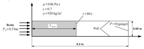
Fig. 2 - Computational domain for the rectilinear solution sumiu um "." de 0.06
