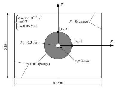
Fig. 3 - Computational domain for the radial 2D solution
