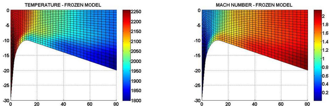
Figure 6. Temperature and Mach number distribution along the nozzle for the frozen model.
