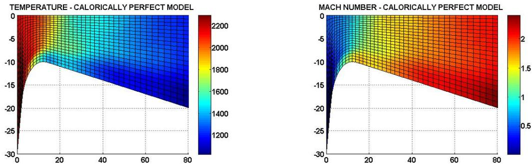
Figure 5. Temperature and pressure distributions along the nozzle for the calorically perfect model.
