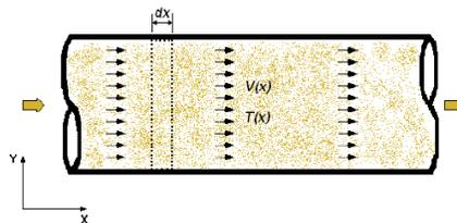
Figure 4. Plug flow reactor model (Leite, 2006).
