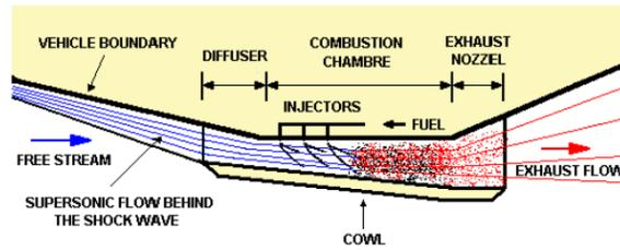
Figure 1. Schematic drawing of a scramjet engine (Curran, 1996).
