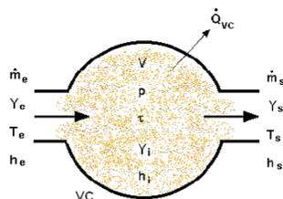
Figure 3. Perfect stirred reactor model (Leite, 2006).
