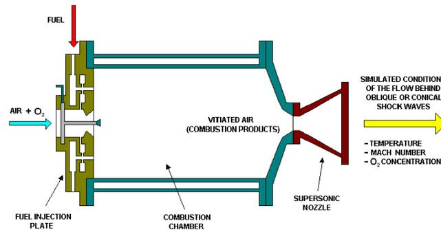
Figure 2. Schematic drawing of a vitiated air generator with supersonic nozzle (Leite et al, 2007).
