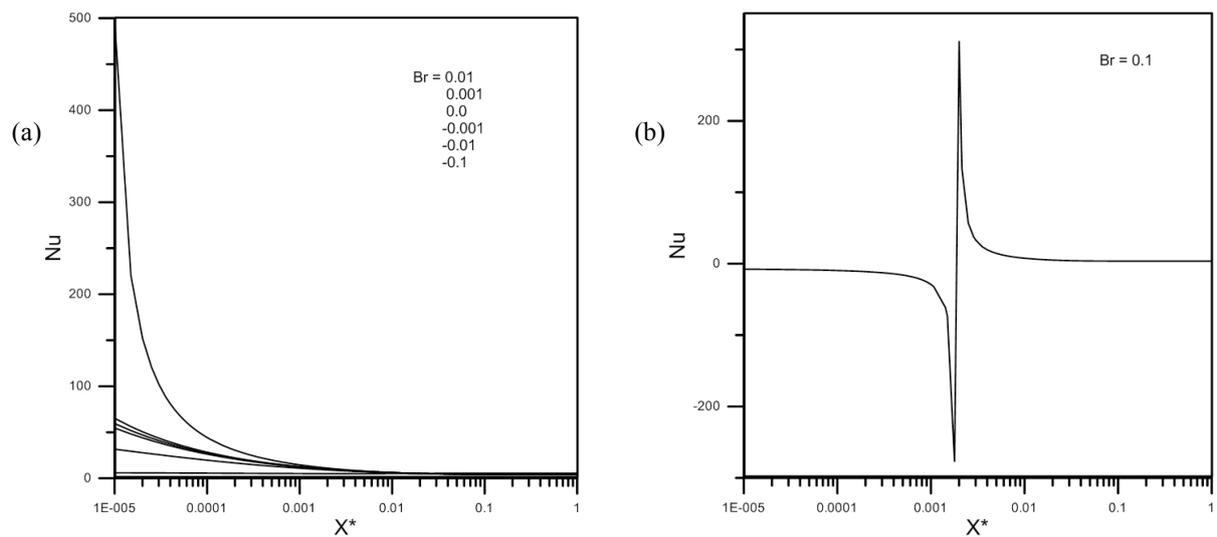
Figure 3. Effect of Brinkman number on Nusselt number for the constant wall heat flux ( $n = 1$ : Newtonian fluid).
