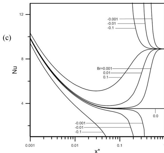
Figure 1. Effect of Brinkman number on Nusselt number for the constant wall temperature (a)  $n = 0.5$ : pseudoplastic fluid; (b)  $n = 1$ : Newtonian fluid; and (c)  $n = 1.5$ : dilatant fluid.
