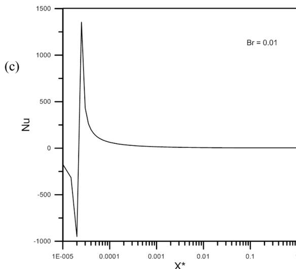
Figure 4. Effect of Brinkman number on Nusselt number for the constant wall heat flux (  $n = 1.5$ : dilatant fluid).
