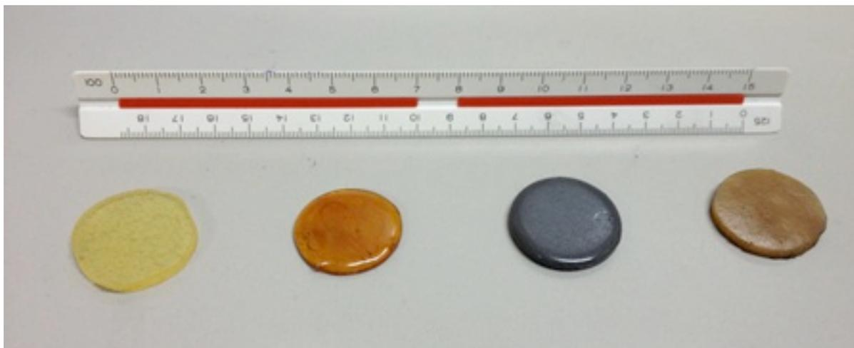
Figure 1. From left to right, phantoms made of: PVC-P, PVC-P and SiO<sub>2</sub> nanoparticles, PVC-P and thermal paste, PVC-P and TiO<sub>2</sub> nanoparticles
