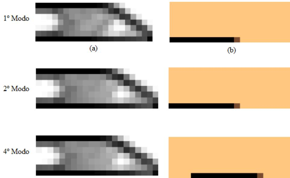
Figure 2: Optimal topologies for distribution of material solid (a) and distribution of piezoelectric material (b) for 1st, 2nd and 4th vibration modes.
