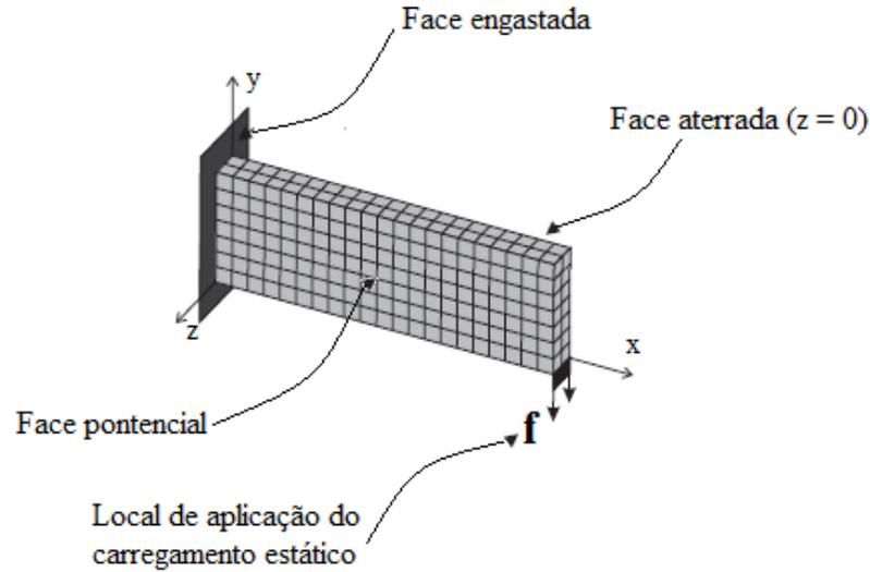
Figure 1 - Cantilever beam discretized in 294 solid isoparametric finite elements.
