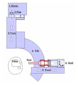
Figure.3: Kinematic configuration of the active manipulator
