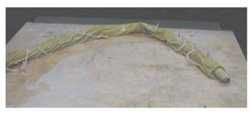
Figure 3: A balloon deployed in a latex 'colon'.
