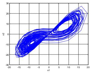
Figure 1: The  $x_1x_2$  phase plan of Lorenz system.
