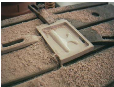
Figure 8. result of the manufacturing process by robot milling.
