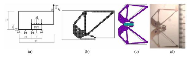
Figure 6. (a) initial design domain; (b) optimal topology; (c) deformed of the optimal topology and (d) manufactured actuator (1 division/mm).
