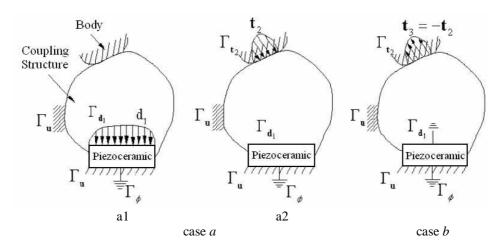
Figure 1. Load cases for calculation of the mean transduction (case a) and mean compliance (case b).
