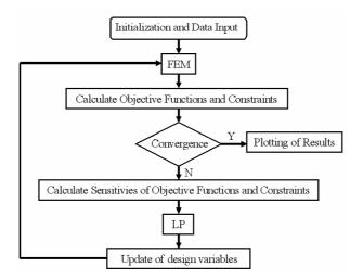
Figure 2. Flowchart of the optimization iterative process.
