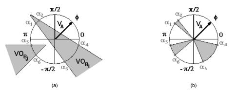
Figure 8. *BOA* Procedure: (a) two obstacles represented by two  $VO_{BS}$  ( $VO_{Bi}$  and  $VO_{Bj}$ ). (b) Velocity Space and the 3 *dangerous velocity direction* sets obtained.
