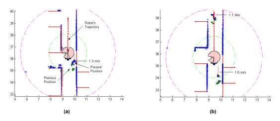
Figure 11. *BOA* Procedure: illustration of the *DVD* sets (salmon areas), laser data (blue dots), environment map (red lines) a person walking close to MOPS at 1.3 m/s (a) and 2 persons walking close to MOPS at 1.1 m/s and 1.6 m/s (b).
