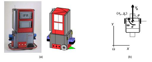
Figure 1. The mobile robot used (a) MOPS and its MatLab model and (b) its kinematic model: Ω is the global coordinate system.
