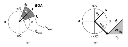
Figure 6. BOA Procedure: (a) the circle of radius  $||V_A||$  represents the velocity space and the dark gray area limited by  $\phi_l$ ,  $\phi_r$ ,  $V_{Amax}$ , and  $V_{Amin}$  represents the set of *reachable velocities*. (b) The use of  $VO_{Bi}$  to calculate the *dangerous velocities*.
