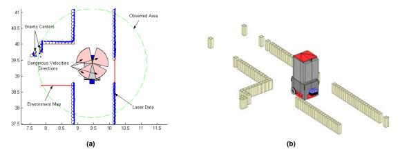
Figure 10. *BOA* Procedure (a): illustration of the *DVD* sets (salmon areas), laser data (blue dots), environment map (red lines), the unmatched obstacles gravity center (red filled circles) and the observed area (green circle). 3-D illustration of the MOPS vicinity (b).
