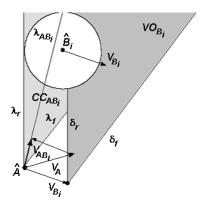
Figure 3. Velocity Obstacle Approach: VO<sub>Bi</sub>.
