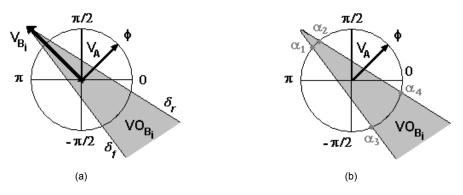
Figure 7. BOA Procedure: (a) and (b) the dangerous velocity direction calculus in the velocity space.
