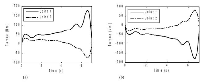
Figure 6. A choice of torque profile that lead (a) robot 1 and (b) robot 2 end-effectors to target position.
