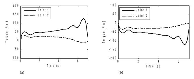
Figure 8. The optimal torque profile that lead (a) robot 1 and (b) robot 2 end-effectors to optimal target position.
