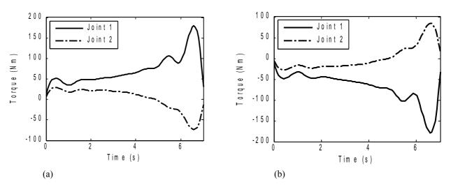
Figure 7. A choice of torque profile that lead (a) robot 1 and (b) robot 2 end-effectors to target position with minimal torque.
