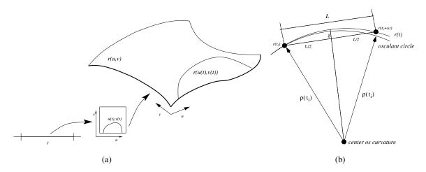
Figure 5. A path r(u(t),v(t)) on the surface S(u,v) (a), and the manufacturing parameters (b).
