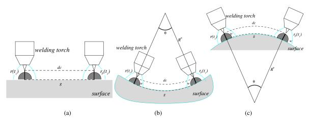
Figure 7. The g variation according the curvature radius  $R^*$ .
