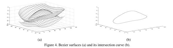
Therefore, applying recursively the method of subdividing patches all area eroded can be localized by this algorithm. It is necessary to identify all curves and to delimitate the area where the welding process have to perform to recover the surface at all. The next step is to compute the curve path that has to be followed by robot's end effector to accomplish the welding task.
