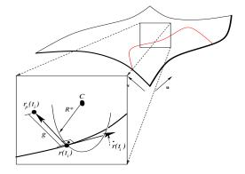
Figure 6. Geometric relationships to compute a parallel path.
