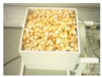
Figure 1. Moisture Sensor final mechanical conception(Lagares and Sousa, 2006)
