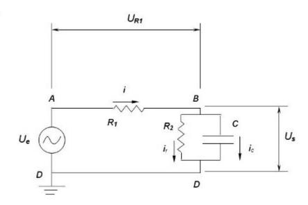
Figure 2. Eletrical circuit used in the moisture measurer
