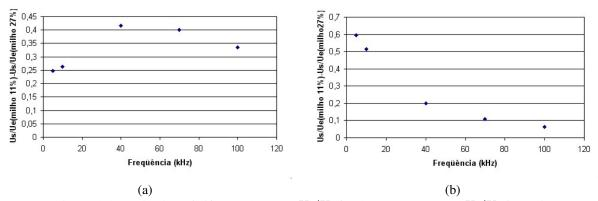
Figure 8. Experimental determination of difference between  $U_s/U_e$  for dry corn (11%) and  $U_s/U_e$  for moist corn (27%): (a)  $R_1$  equal to  $10k\Omega$  (b)  $R_1$  equal to  $100k\Omega$
