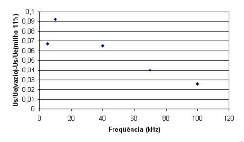
Figure 9. Diference between  $U_s/U_e$  for empty sensor and  $U_s/U_e$  for dry corn (11%)
