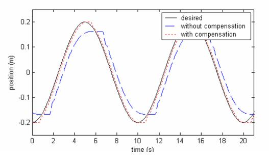
Figure 4. Experimental results to sinusoidal trajectory tracking
