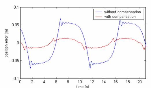
Figure 6. Position error to sinusoidal trajectory
