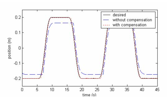
Figure 5. Experimental results to polynomial trajectory tracking
