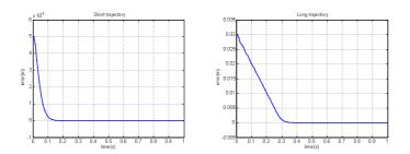
Figure 6 – Position error: short and long trajectories
