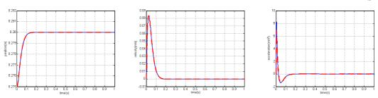
Figure 12 - Comparison between position, velocity and acceleration (blue lines) and the corresponding observer estimated values (red dashed line) – short trajectory
