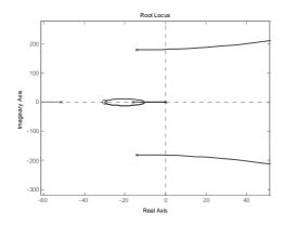
Figure 22 - Root locus with augmented system and a 30 rad/s filter
